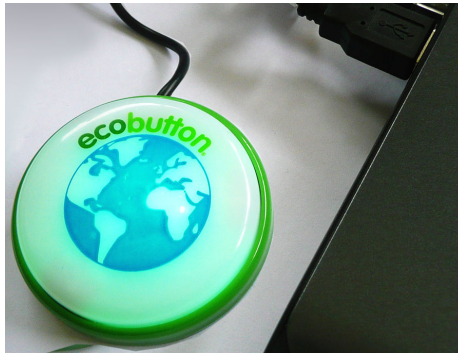
Figure 3: Ecobutton is a USB device allowing a computer to be put into a low-power mode very simply
