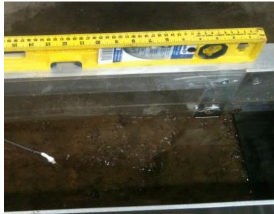
Fig. 4: Photograph showing the inlet pool and the first embedded sensor. The surface flow sensor is not installed at this time.
