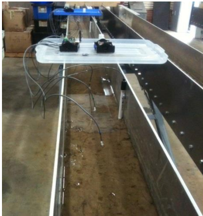
Fig. 3: Photograph of fluvium showing sensor positions.
