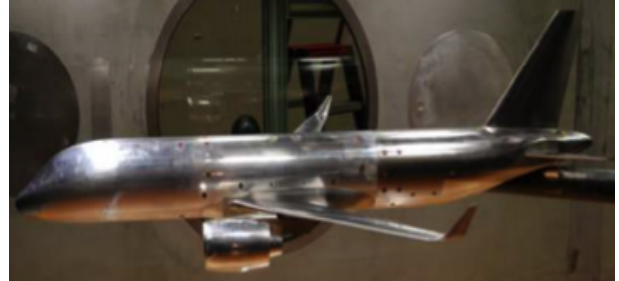
Fig. 1 Wind tunnel model of the regional jet aircraft in scale 1:23
