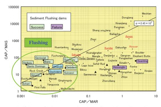
**Figure 9.** Plot of flushing projects from diverse environments showing that successful cases are characterized by impoundment ratios of 0.4 or less. That is, reservoir storage capacity divided by mean annual runoff (inflow to the reservoir) should be less than 0.4.
