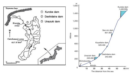
Figure 12. Kurobe River, Japan. Map of drainage basin and location of major reservoirs (a), and longitudinal profile showing all reservoirs (b).
