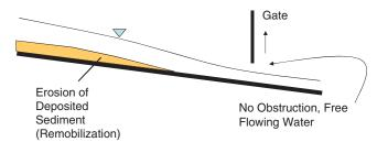
Figure 8. Schematic representation of drawdown flushing.
