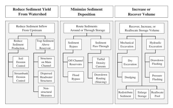
Figure 1. Classification of strategies for sediment management from the perspective of sustaining reservoir capacity.
