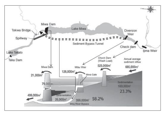
Figure 3. Diagram of sediment bypass system for Miwa Dam, Mibu River, Japan. A check dam traps coarse sediment, and a diversion weir diverts flows with high suspended sediment concentrations into a bypass tunnel.
