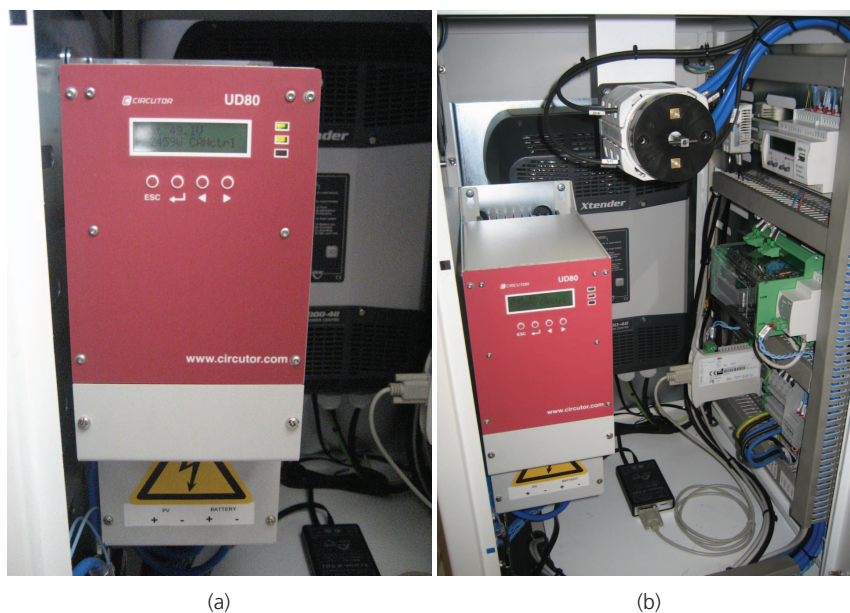
Figure 5. Prototype of the power conditioning system developed within the Zerowin project. The figure shows the charge controller, and the charge controller and supervisory controller situated inside the cabinet (Arranz et al. , 2012)
