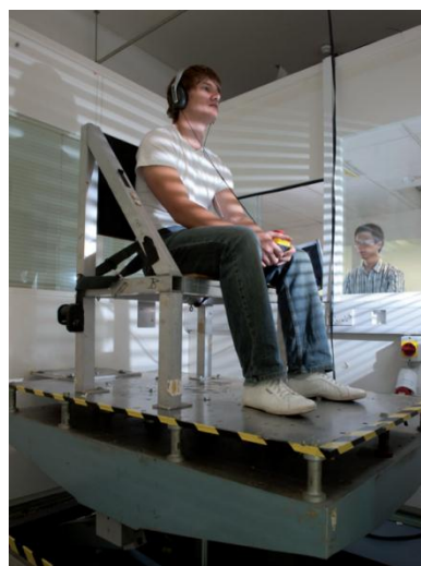
Figure 3.1 One-meter vertical electro-hydraulic vibrator. From http://www.southampton.ac.uk/hfru/lab_facilities/vertical_vibrator.html
