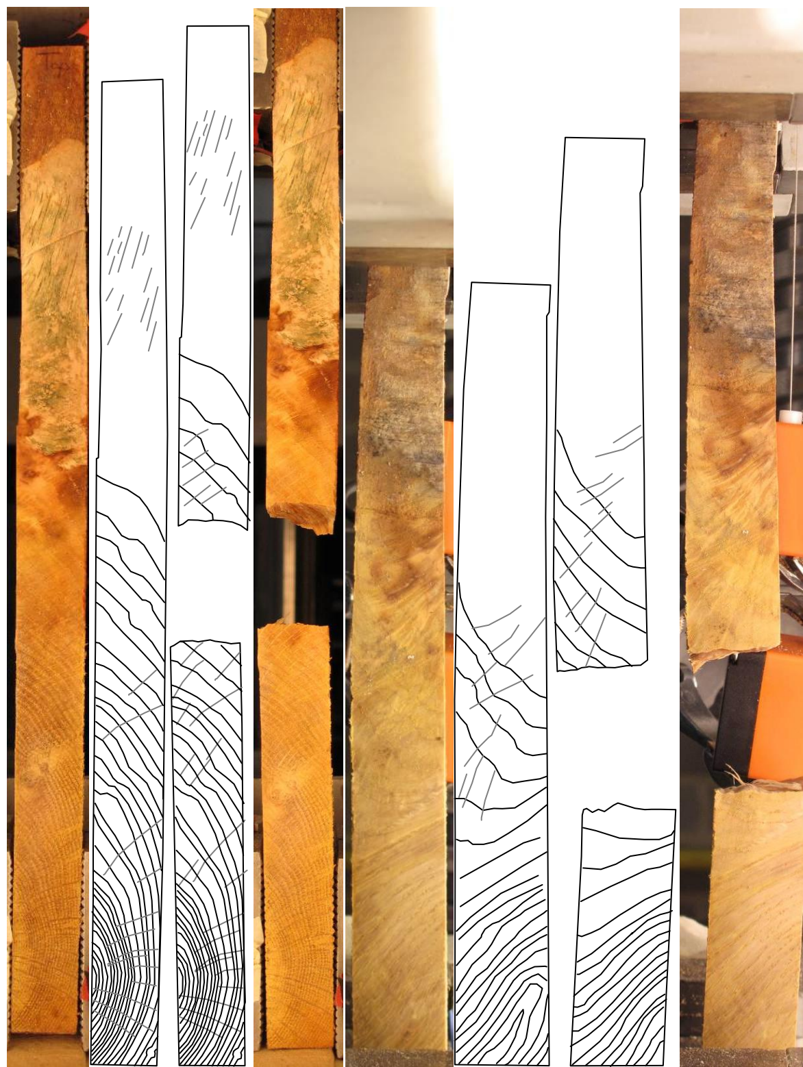
FIGURE 405: SAMPLE GRAIN ORIENTATIONS OF THE FRONT (LEFT 4 IMAGES) AND SIDE (RIGHT 4 IMAGES) VIEW BEFORE (FIRST 2 OF 4 IMAGES) AND AFTER (LAST 2 OF 4 IMAGES) BREAKAGE
