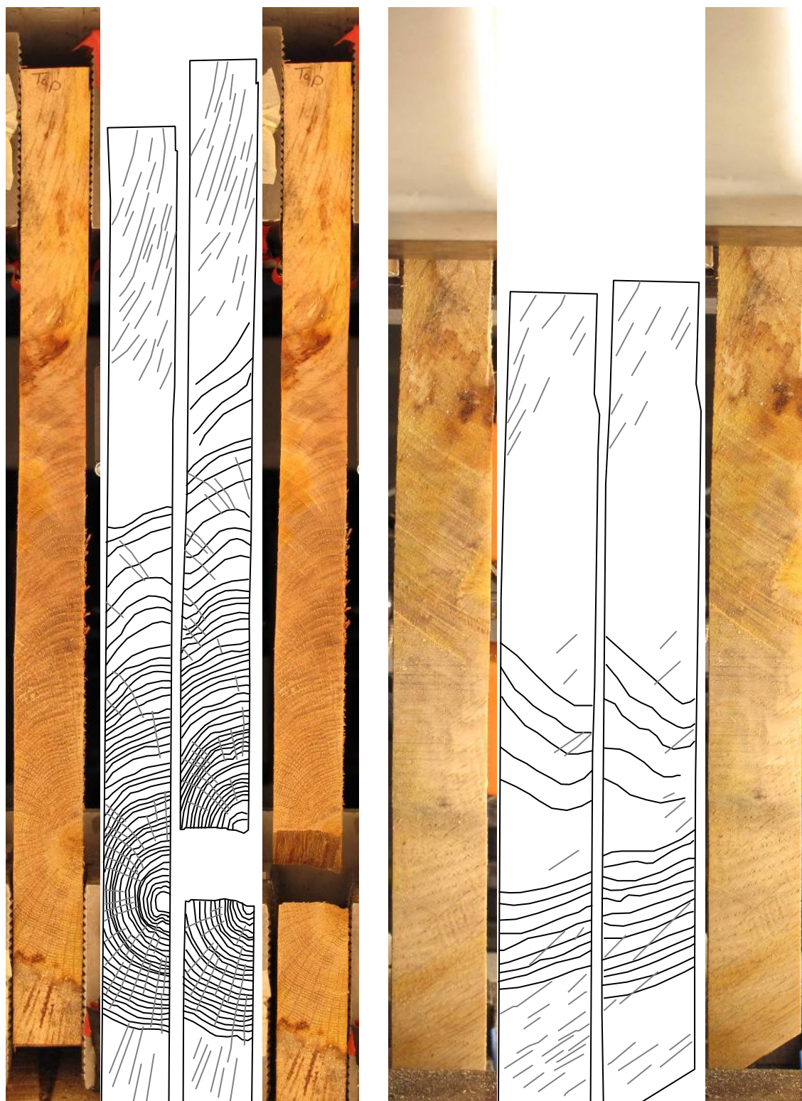
FIGURE 294: SAMPLE GRAIN ORIENTATIONS OF THE FRONT (LEFT 4 IMAGES) AND SIDE (RIGHT 4 IMAGES) VIEW BEFORE (FIRST 2 OF 4 IMAGES) AND AFTER (LAST 2 OF 4 IMAGES) BREAKAGE
