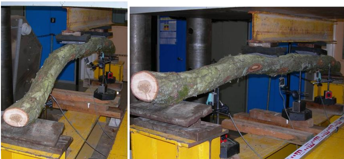
FIGURE 79: PRE LOAD SET-UP AND SAMPLE AFTER FAILURE (LEFT TO RIGHT)
