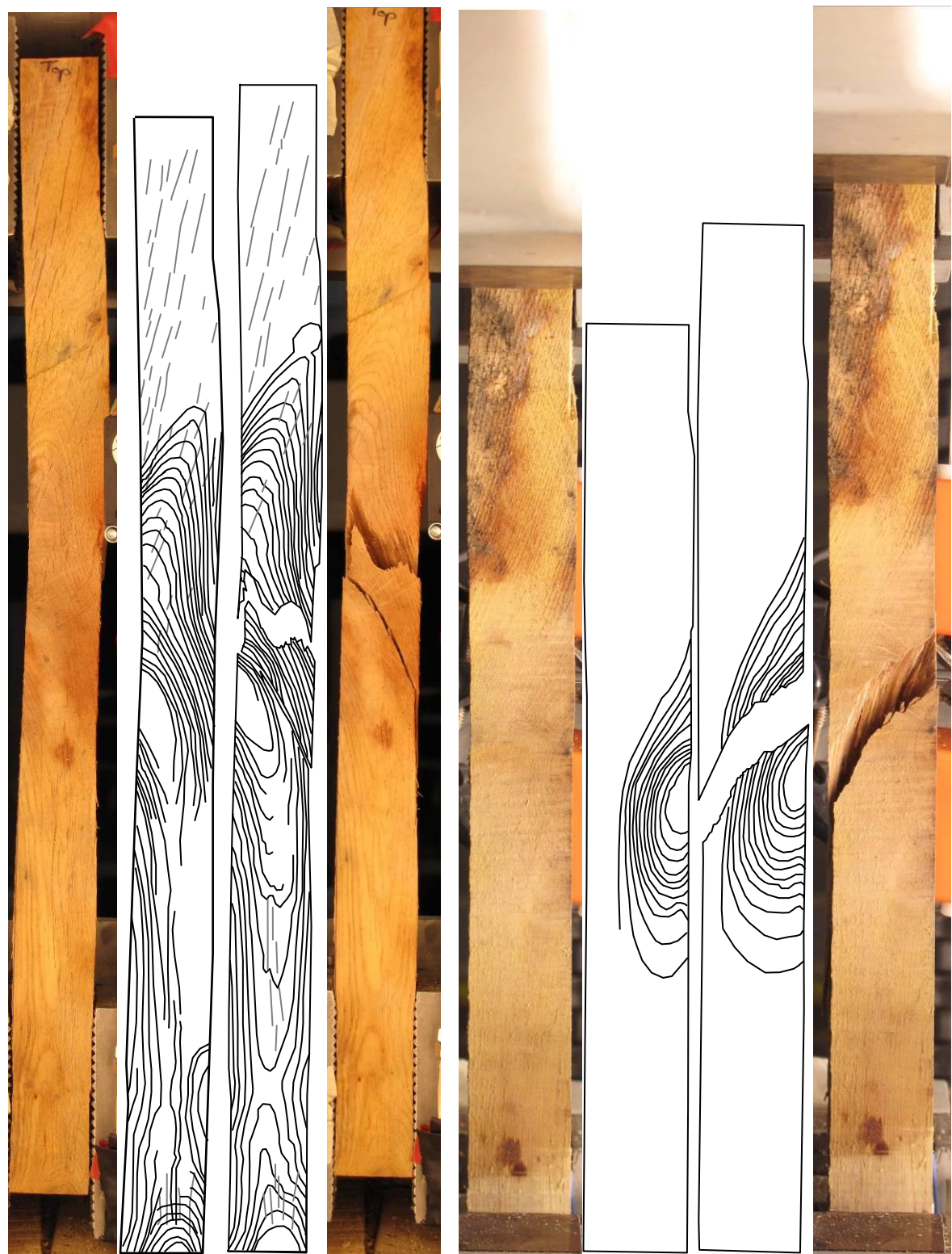
FIGURE 109: SAMPLE GRAIN ORIENTATIONS OF THE FRONT (LEFT 4 IMAGES) AND SIDE (RIGHT 4 IMAGES) VIEW BEFORE (FIRST 2 OF 4 IMAGES) AND AFTER (LAST 2 OF 4 IMAGES) BREAKAGE
