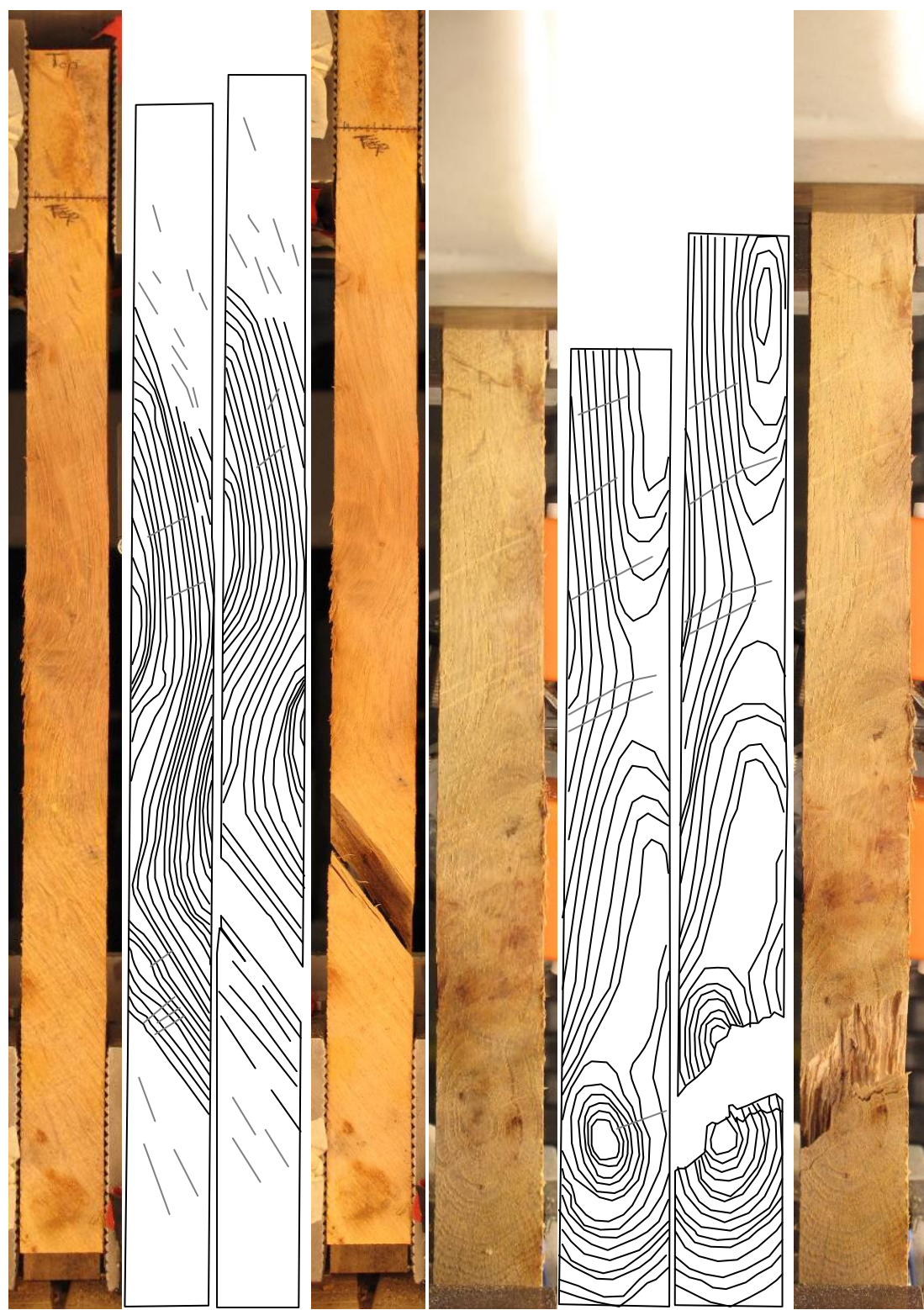
FIGURE 331: SAMPLE GRAIN ORIENTATIONS OF THE FRONT (LEFT 4 IMAGES) AND SIDE (RIGHT 4 IMAGES) VIEW BEFORE (FIRST 2 OF 4 IMAGES) AND AFTER (LAST 2 OF 4 IMAGES) BREAKAGE
