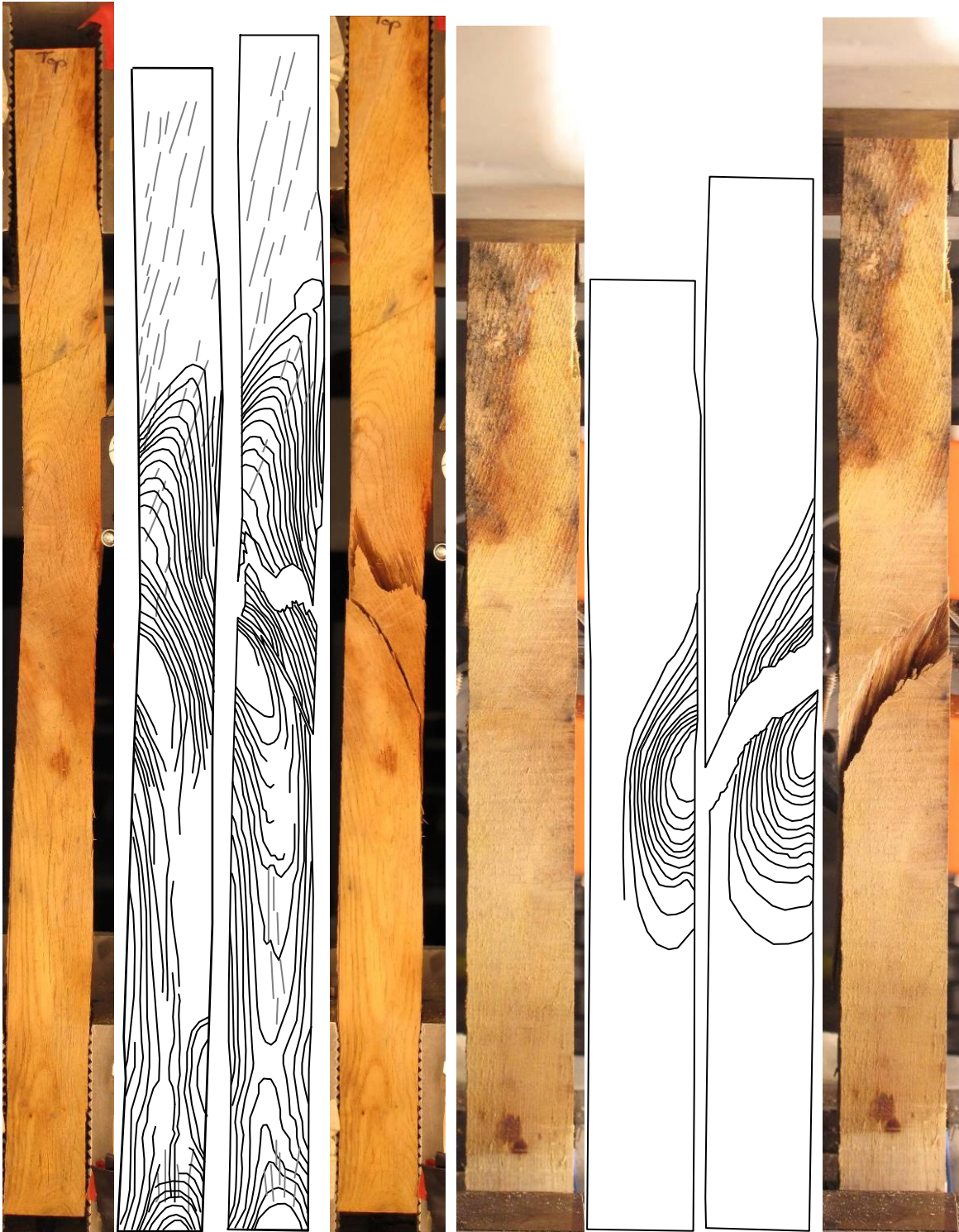
FIGURE 56: G1 SAMPLE GRAIN ORIENTATIONS OF THE FRONT VIEW (LEFT 4 IMAGES) AND SIDE VIEW (RIGHT 4 IMAGES); WITH FIRST 2 OF 4 IMAGES BEFORE FAILURE AND LAST 2 OF 4 IMAGES AFTER FAILURE
