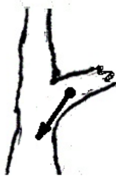
FIGURE 17: TREE JOINT SHOWING THE BRANCH'S CENTRE OF MASS IS DIRECTED TOWARDS THE BASE OF THE CONNECTION
