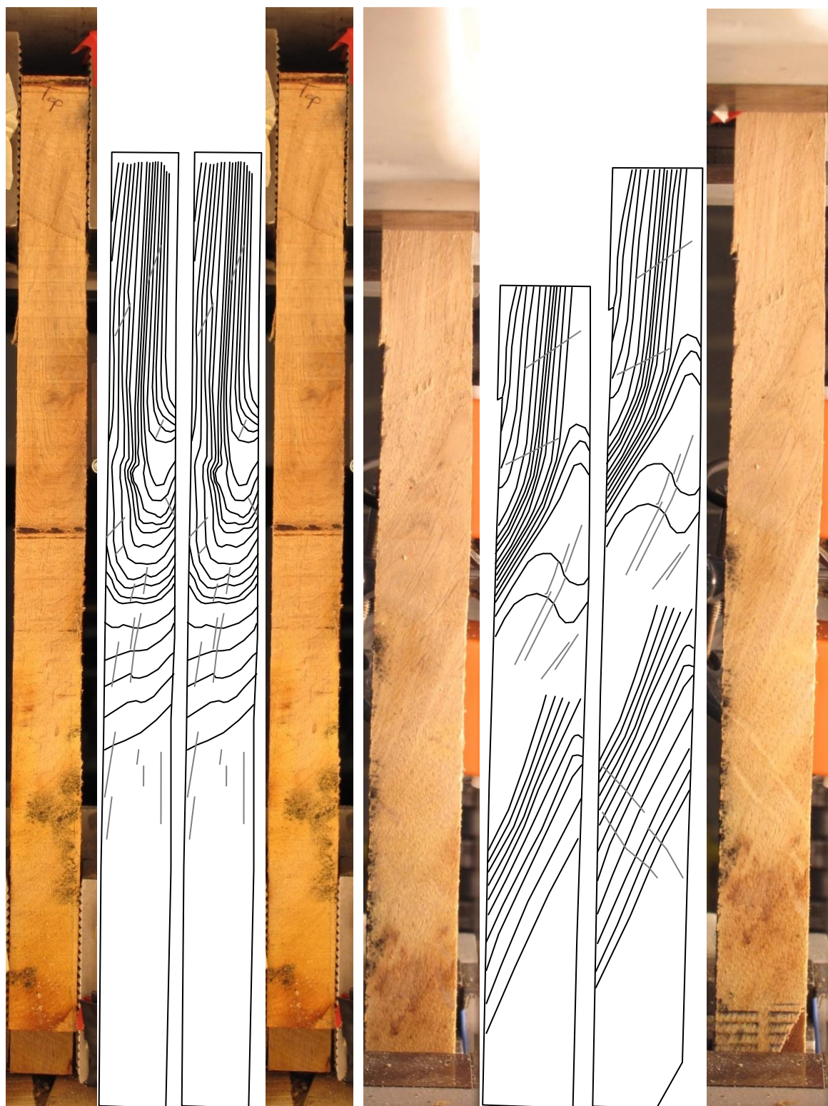
FIGURE 747: SAMPLE GRAIN ORIENTATIONS OF THE FRONT (LEFT 4 IMAGES) AND SIDE (RIGHT 4 IMAGES) VIEW BEFORE (FIRST 2 OF 4 IMAGES) AND AFTER (LAST 2 OF 4 IMAGES) BREAKAGE
