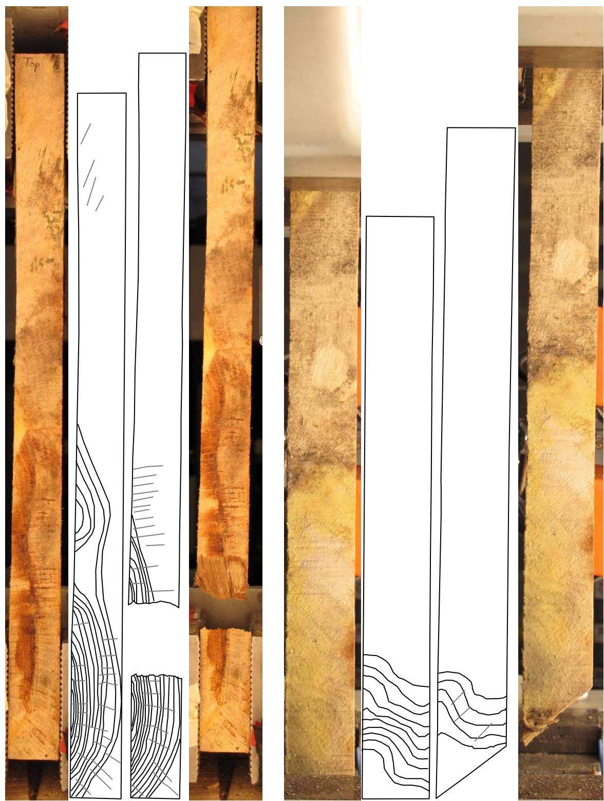
FIGURE 257: SAMPLE GRAIN ORIENTATIONS OF THE FRONT (LEFT 4 IMAGES) AND SIDE (RIGHT 4 IMAGES) VIEW BEFORE (FIRST 2 OF 4 IMAGES) AND AFTER (LAST 2 OF 4 IMAGES) BREAKAGE
