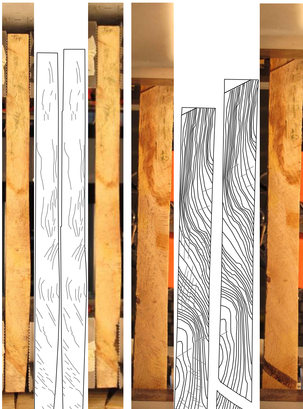
FIGURE 449: SAMPLE GRAIN ORIENTATIONS OF THE FRONT (LEFT 4 IMAGES) AND SIDE (RIGHT 4 IMAGES) VIEW BEFORE (FIRST 2 OF 4 IMAGES) AND AFTER (LAST 2 OF 4 IMAGES) BREAKAGE
