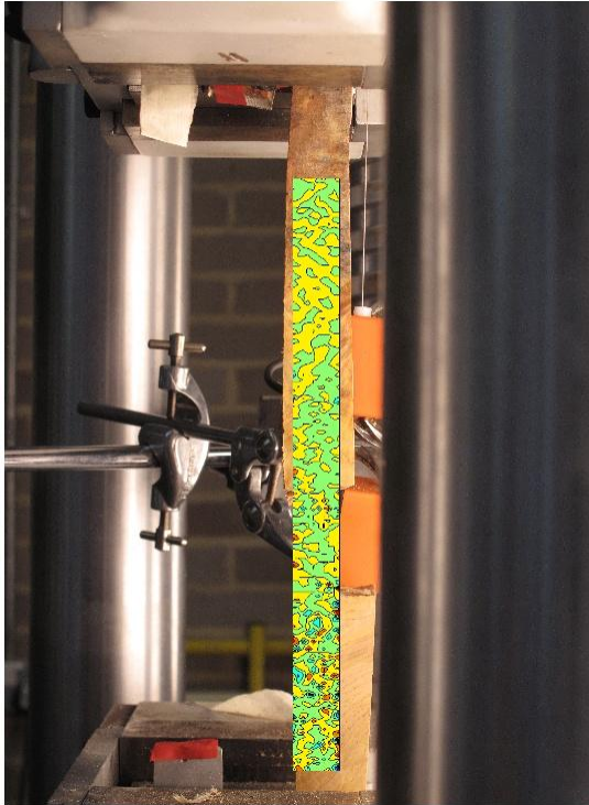
FIGURE 426: X DIRECTION PIV FIRST-LAST DITCH ENGINEERING STRAIN OVER IMAGE
