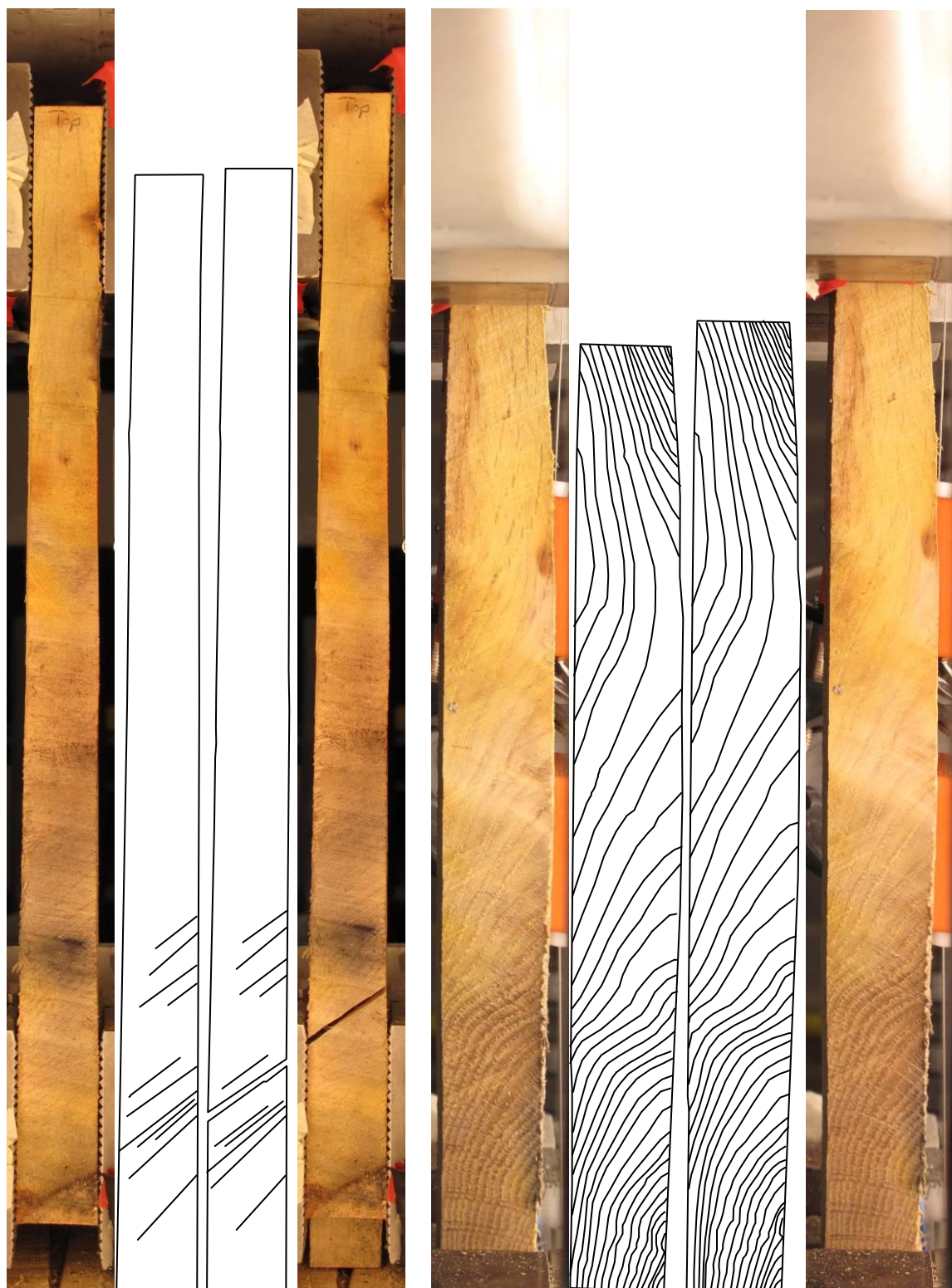
FIGURE 146: SAMPLE GRAIN ORIENTATIONS OF THE FRONT (LEFT 4 IMAGES) AND SIDE (RIGHT 4 IMAGES) VIEW BEFORE (FIRST 2 OF 4 IMAGES) AND AFTER (LAST 2 OF 4 IMAGES) BREAKAGE
