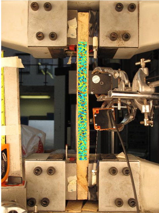
FIGURE 460: Y DIRECTION PIV FIRST-LAST DITCH TRUE STRAIN OVER IMAGE
