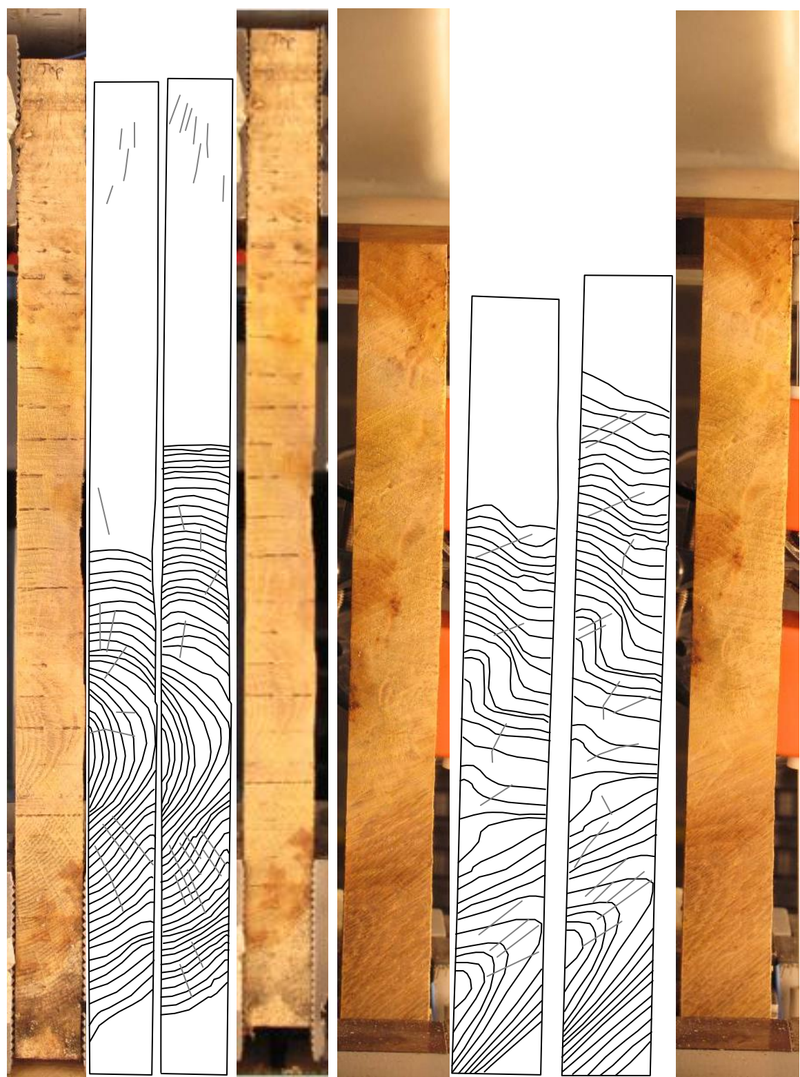
FIGURE 486: SAMPLE GRAIN ORIENTATIONS OF THE FRONT (LEFT 4 IMAGES) AND SIDE (RIGHT 4 IMAGES) VIEW BEFORE (FIRST 2 OF 4 IMAGES) AND AFTER (LAST 2 OF 4 IMAGES) BREAKAGE
