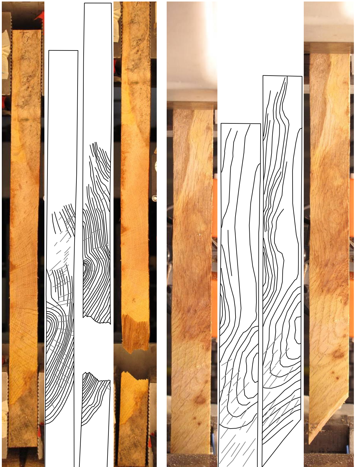
FIGURE 220: SAMPLE GRAIN ORIENTATIONS OF THE FRONT (LEFT 4 IMAGES) AND SIDE (RIGHT 4 IMAGES) VIEW BEFORE (FIRST 2 OF 4 IMAGES) AND AFTER (LAST 2 OF 4 IMAGES) BREAKAGE
