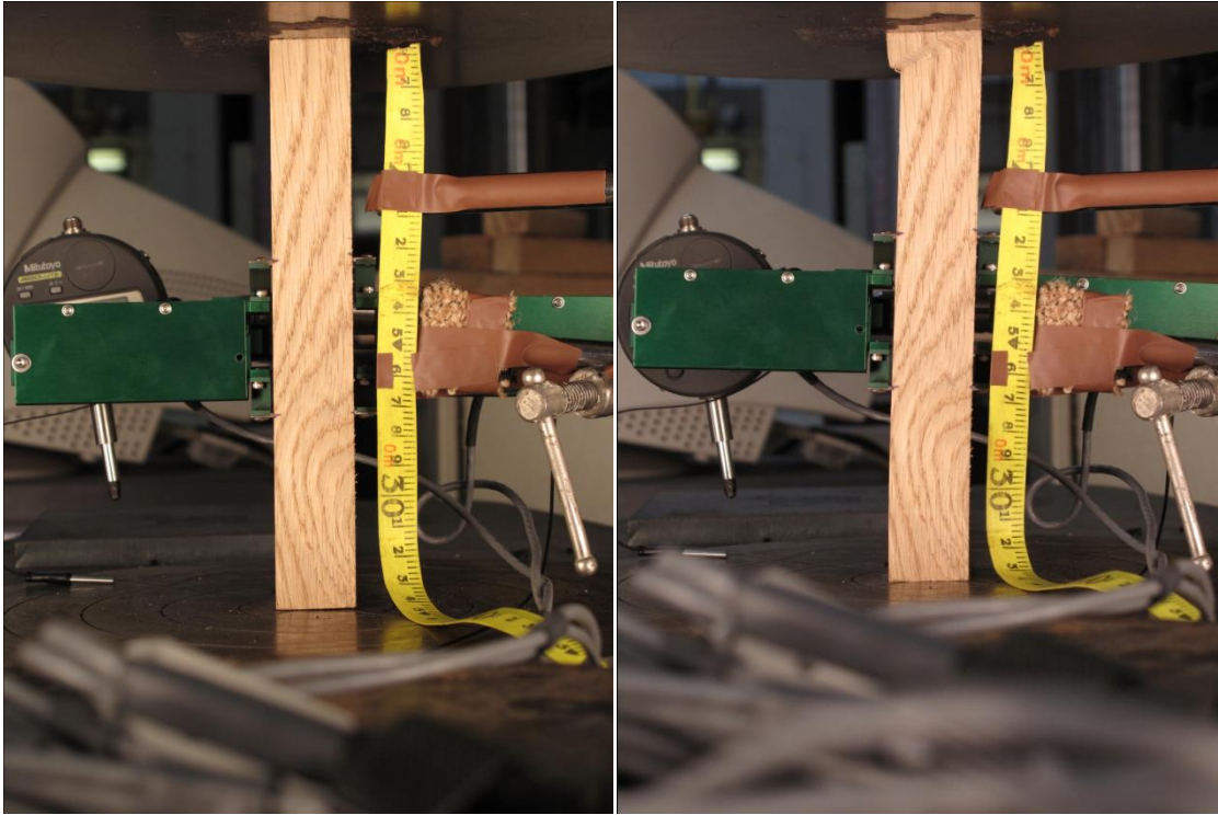
FIGURE 25: COMPRESSION TEST SET-UP VIEW FROM CAMERA OF SAMPLE B2 BEFORE AND AFTER TESTING SHOWING COMPRESSION FAILURE AT THE TOP LEFT OF SAMPLE
