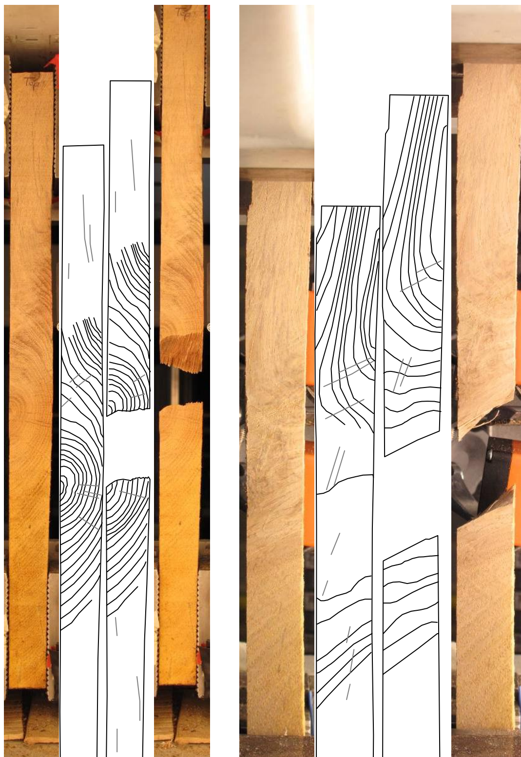
FIGURE 599: SAMPLE GRAIN ORIENTATIONS OF THE FRONT (LEFT 4 IMAGES) AND SIDE (RIGHT 4 IMAGES) VIEW BEFORE (FIRST 2 OF 4 IMAGES) AND AFTER (LAST 2 OF 4 IMAGES) BREAKAGE
