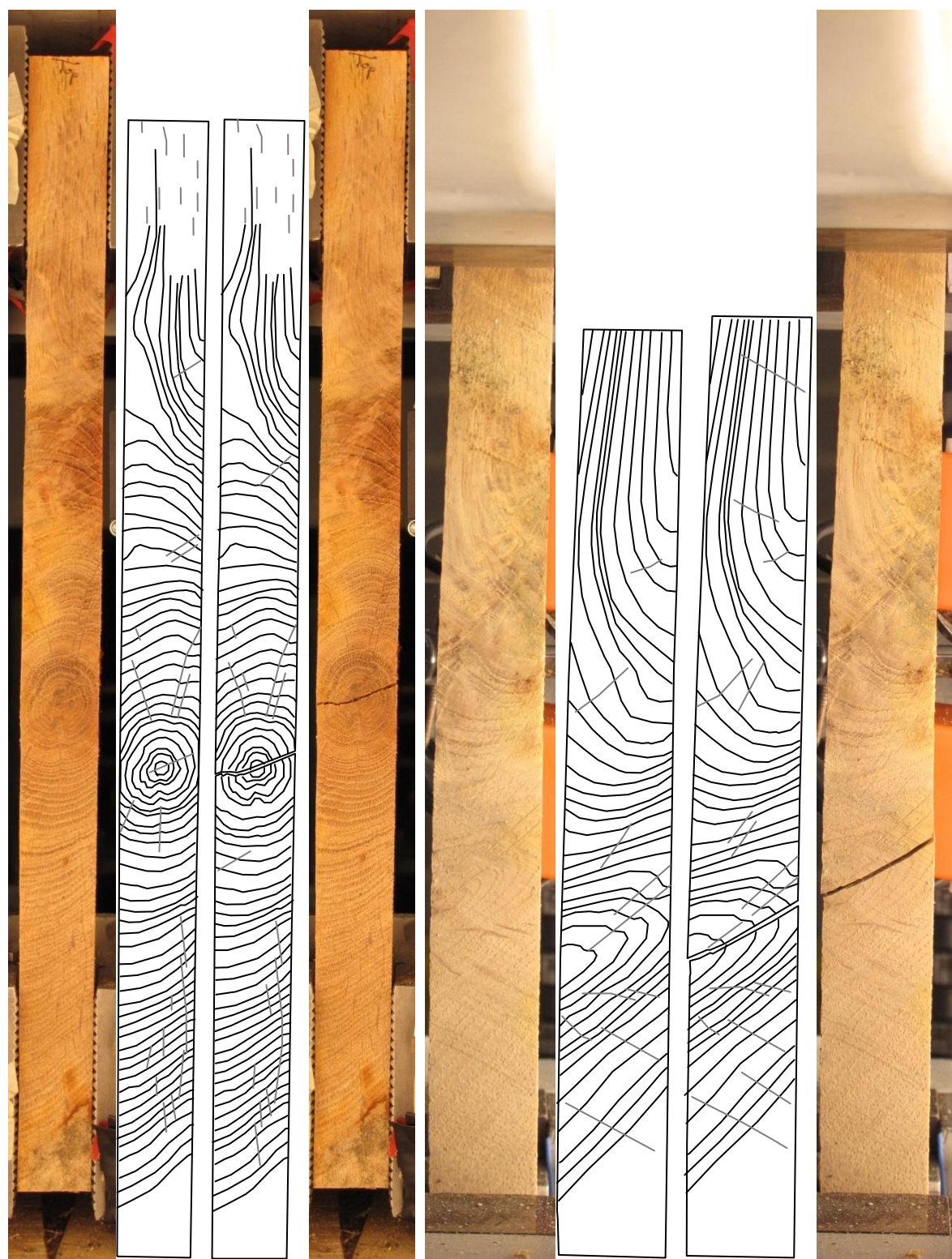
FIGURE 784: SAMPLE GRAIN ORIENTATIONS OF THE FRONT (LEFT 4 IMAGES) AND SIDE (RIGHT 4 IMAGES) VIEW BEFORE (FIRST 2 OF 4 IMAGES) AND AFTER (LAST 2 OF 4 IMAGES) BREAKAGE
