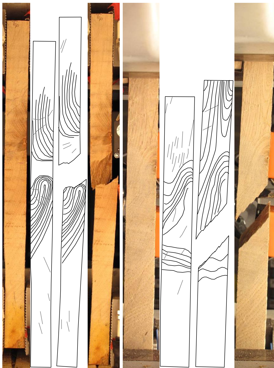
FIGURE 636: SAMPLE GRAIN ORIENTATIONS OF THE FRONT (LEFT 4 IMAGES) AND SIDE (RIGHT 4 IMAGES) VIEW BEFORE (FIRST 2 OF 4 IMAGES) AND AFTER (LAST 2 OF 4 IMAGES) BREAKAGE
