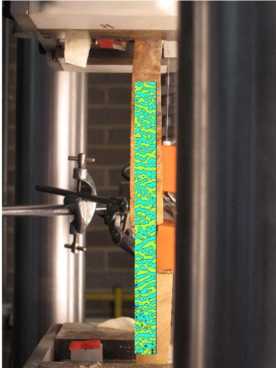
FIGURE 430: Y DIRECTION PIV FIRST-LAST DITCH TRUE STRAIN OVER IMAGE
