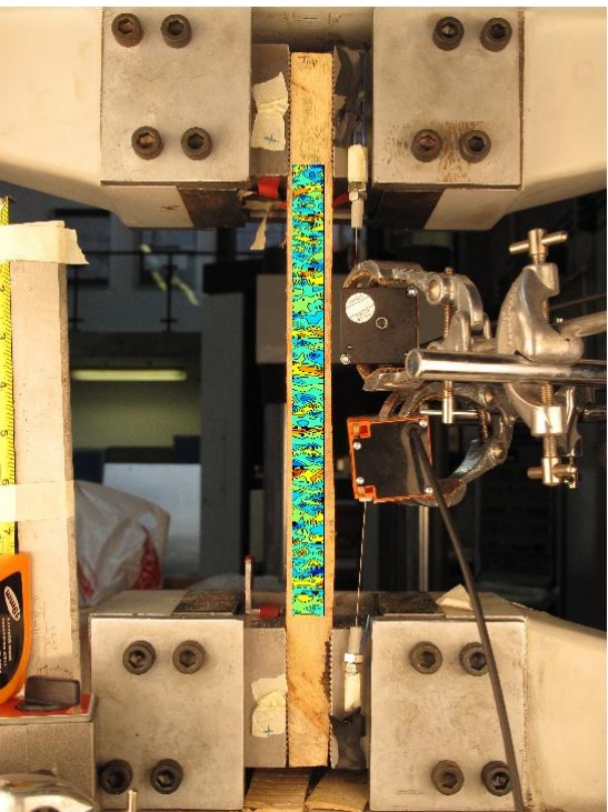
FIGURE 457: Y DIRECTION PIV FIRST-LAST DITCH ENGINEERING STRAIN OVER IMAGE
