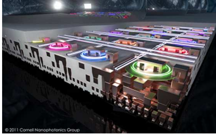
FIGURE 1.1: 3D schematic illustrating the proposed back-end integration of SiP with CMOS technology [31]
