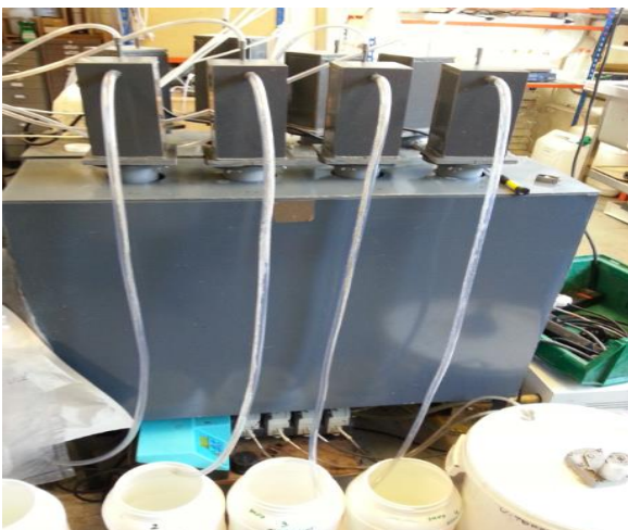
Figure 3.11 Anaerobic filter and UASB digester
