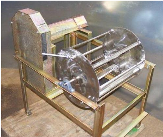
Figure 3.5 Washing machine during construction
