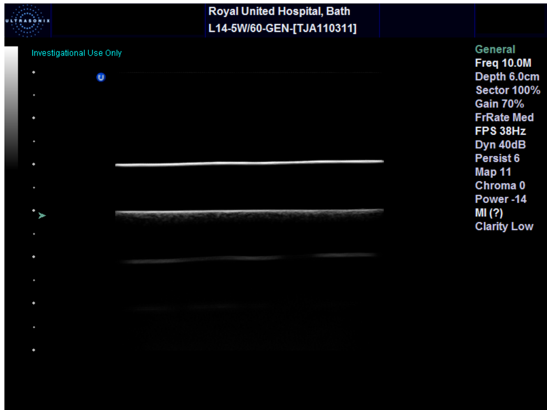
Figure 10.4 Example of image of acoustic polymer inert reflector in MAGIC gel phantom A. The interface between MAGIC gel and acoustic polymer inert reflector is at the level of the focal depth (31mm) as indicated by the blue arrow.
