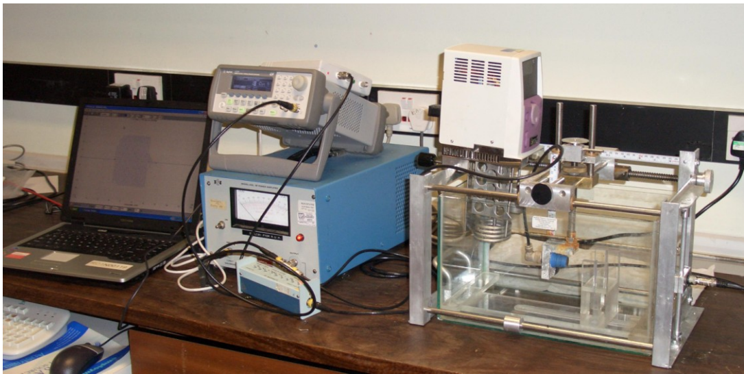
Figure 3.3. Photo of the measurement apparatus for attenuation measurements. The water tank containing the samples is shown on the right of the photograph. The pulse generating system is in the centre, with the laptop used to store the received signals is shown on the left.
