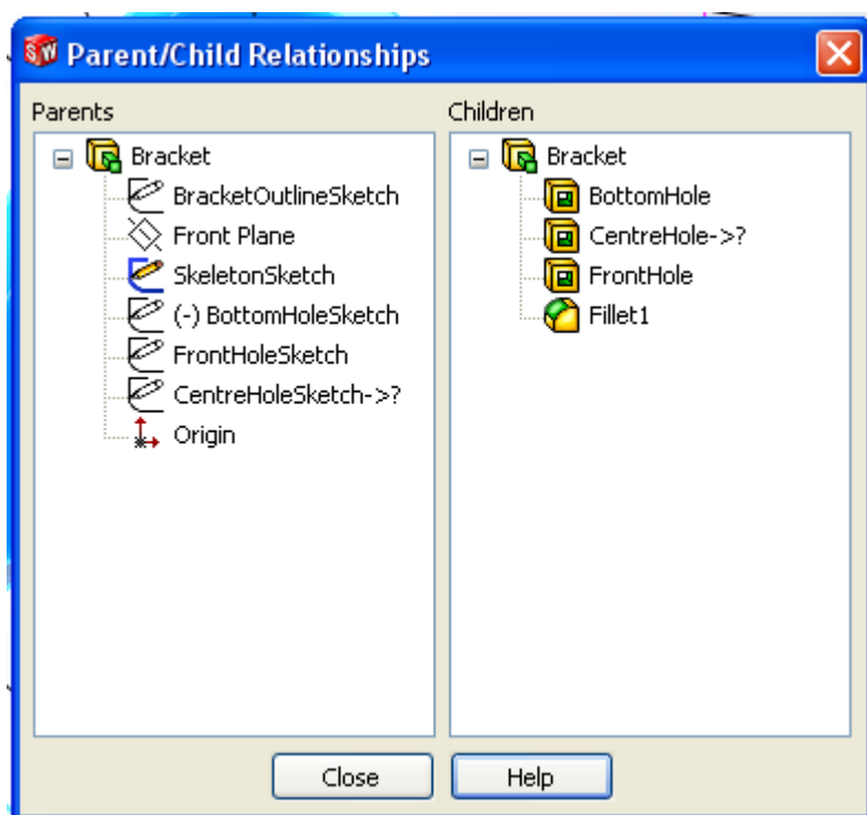
Figure 31 Parent-Child operation dependency display in Solidworks
