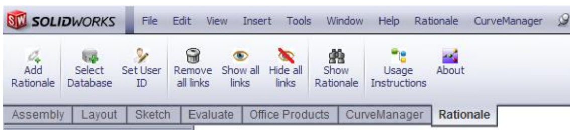
Figure 26 The design rationale toolbar providing access to design rationale linking functionality
