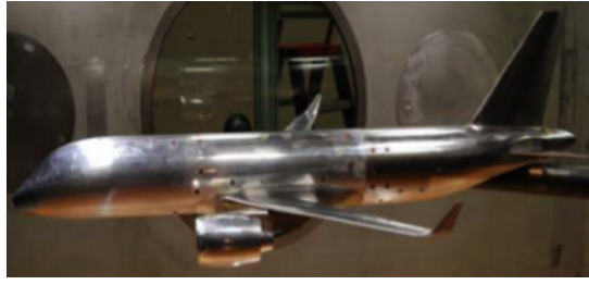
Figure 4.1: Wind tunnel model of the regional jet aircraft in scale 1:23
