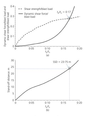
**Figure 4.** (a) Calculation of critical  $t_d/t_n$  ratio for the Murrah Building. (b) Calculation of SSD from the given  $t_d/t_n$  ratio
