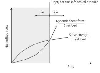
Figure 1. Safe stand-off distance considering shear failure
