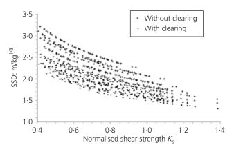
Figure 5. Normalised shear strength plotted against SSD
