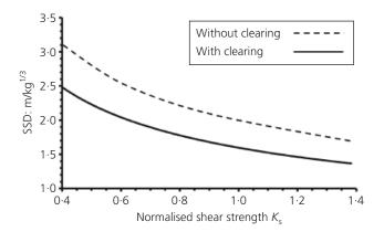
Figure 6. Normalised shear strength plotted against SSD design chart for RC columns
