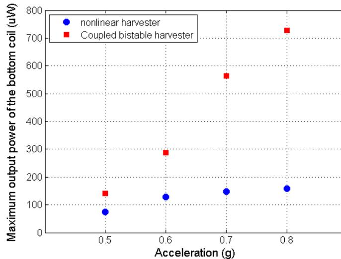
**Figure 6.** Comparisons of output power under various accelerations.
