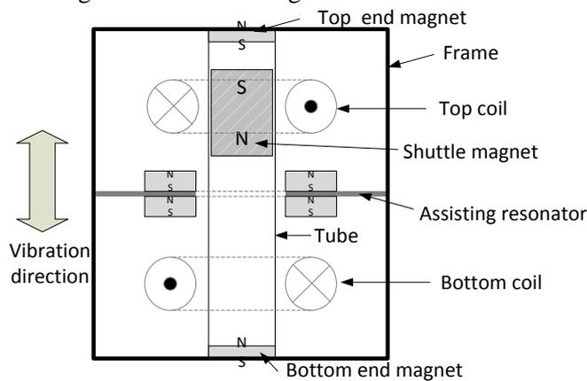
**Figure 1.** Structure of the miniature coupled bistable energy harvester.
