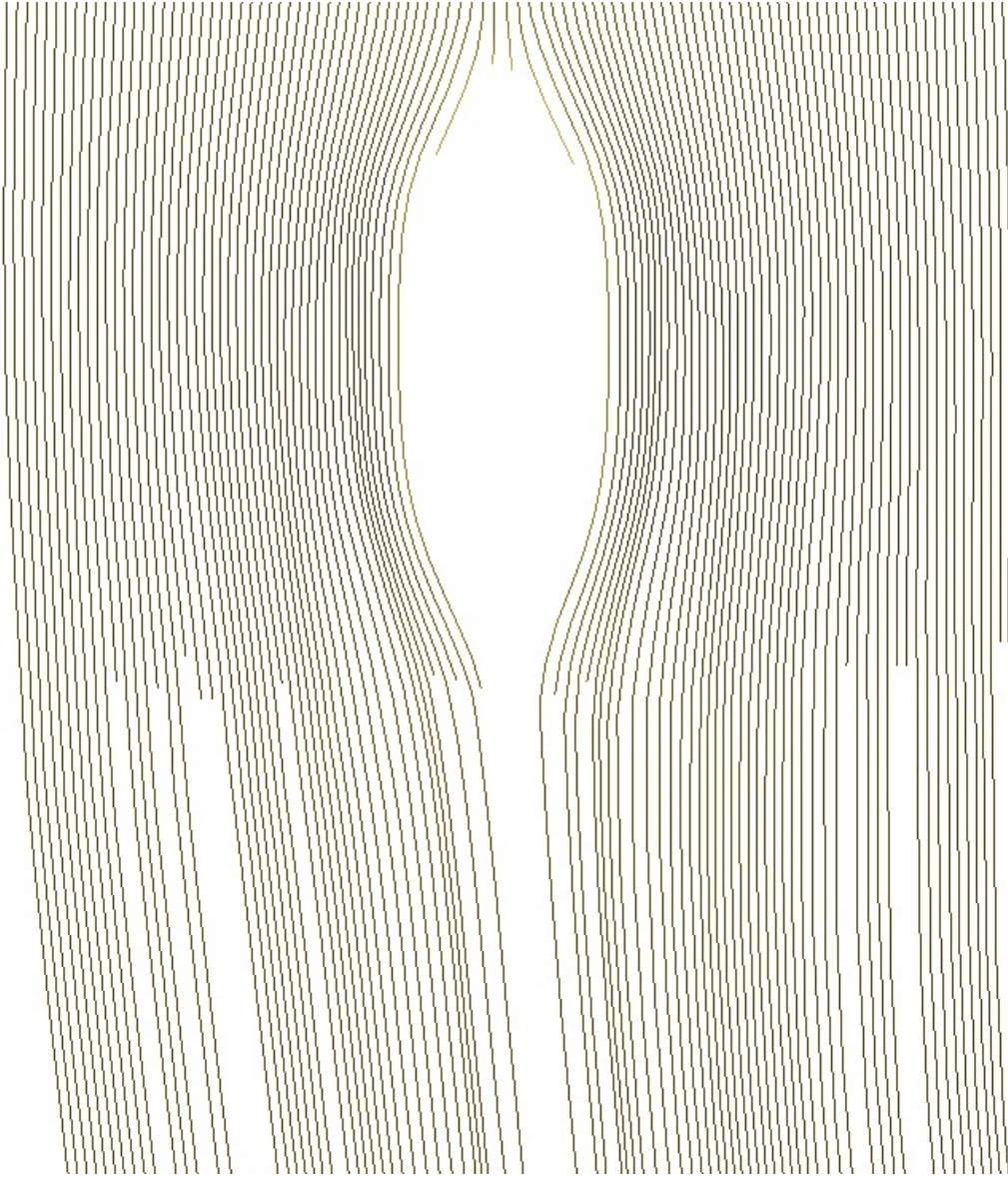
Figure 6.23: Streamlines past stator of 100mm Rim Driven Thruster at 3000 RPM.
