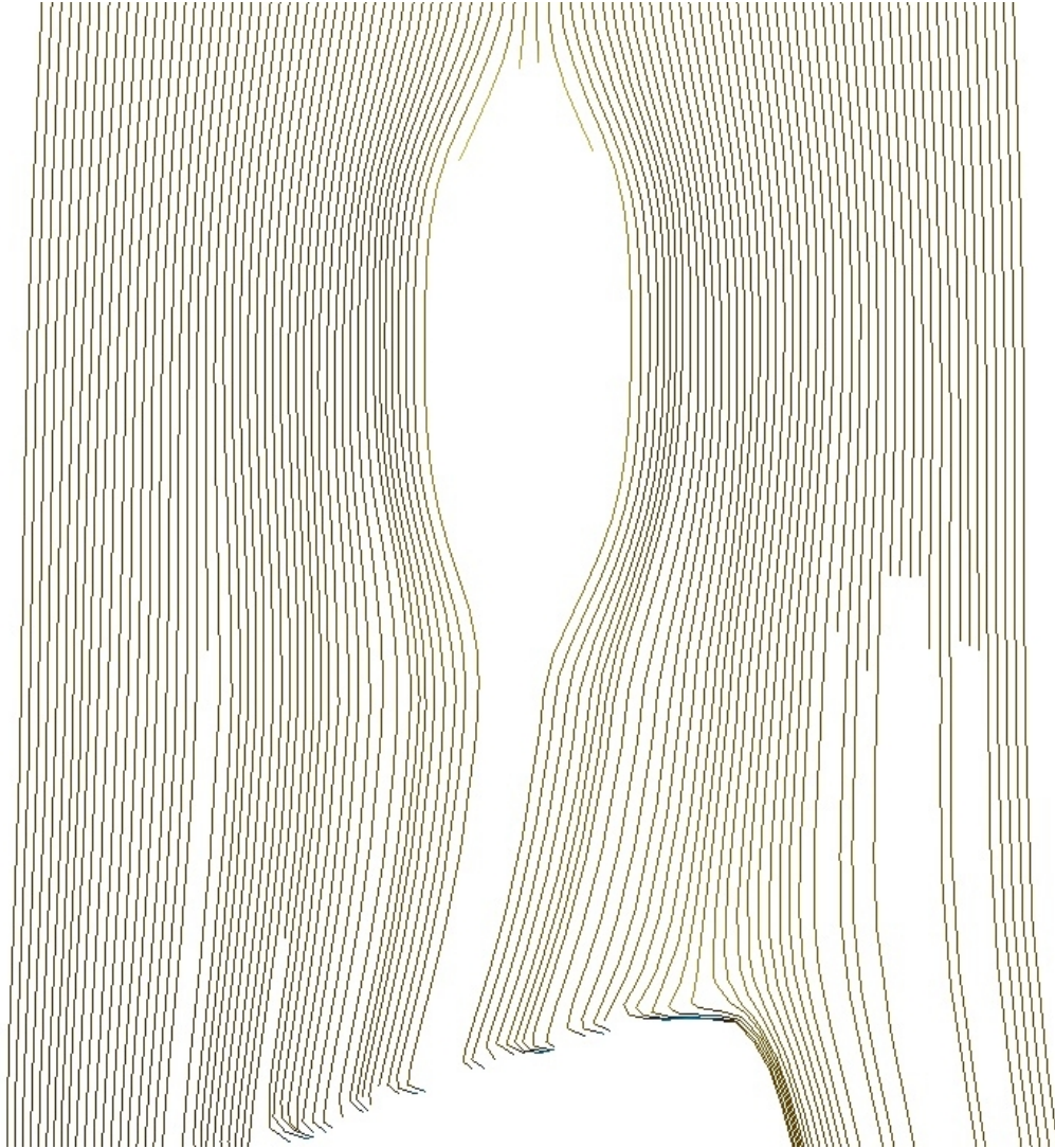
Figure 6.24: Streamlines past stator of 100mm Rim Driven Thruster at 3000 RPM, one half period later.
