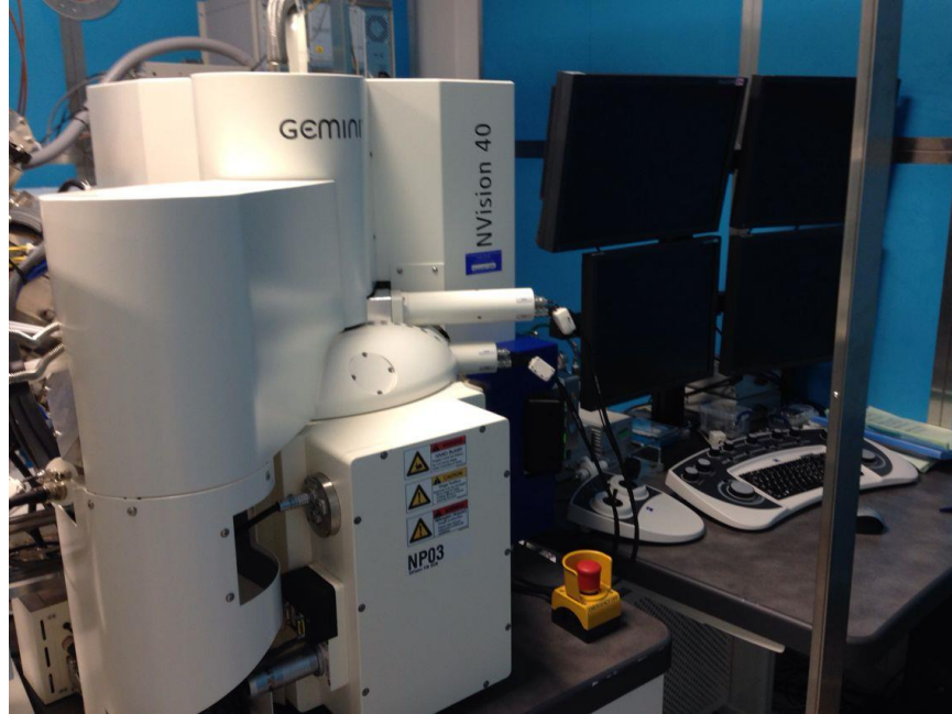
Figure 3-16 Photo of Zeiss NVision 40 CrossBeam FIB System.
