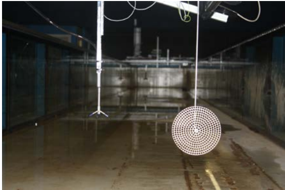
Figure 2. 150mm porous disc rotor simulator and ADV velocity probe to the left.
