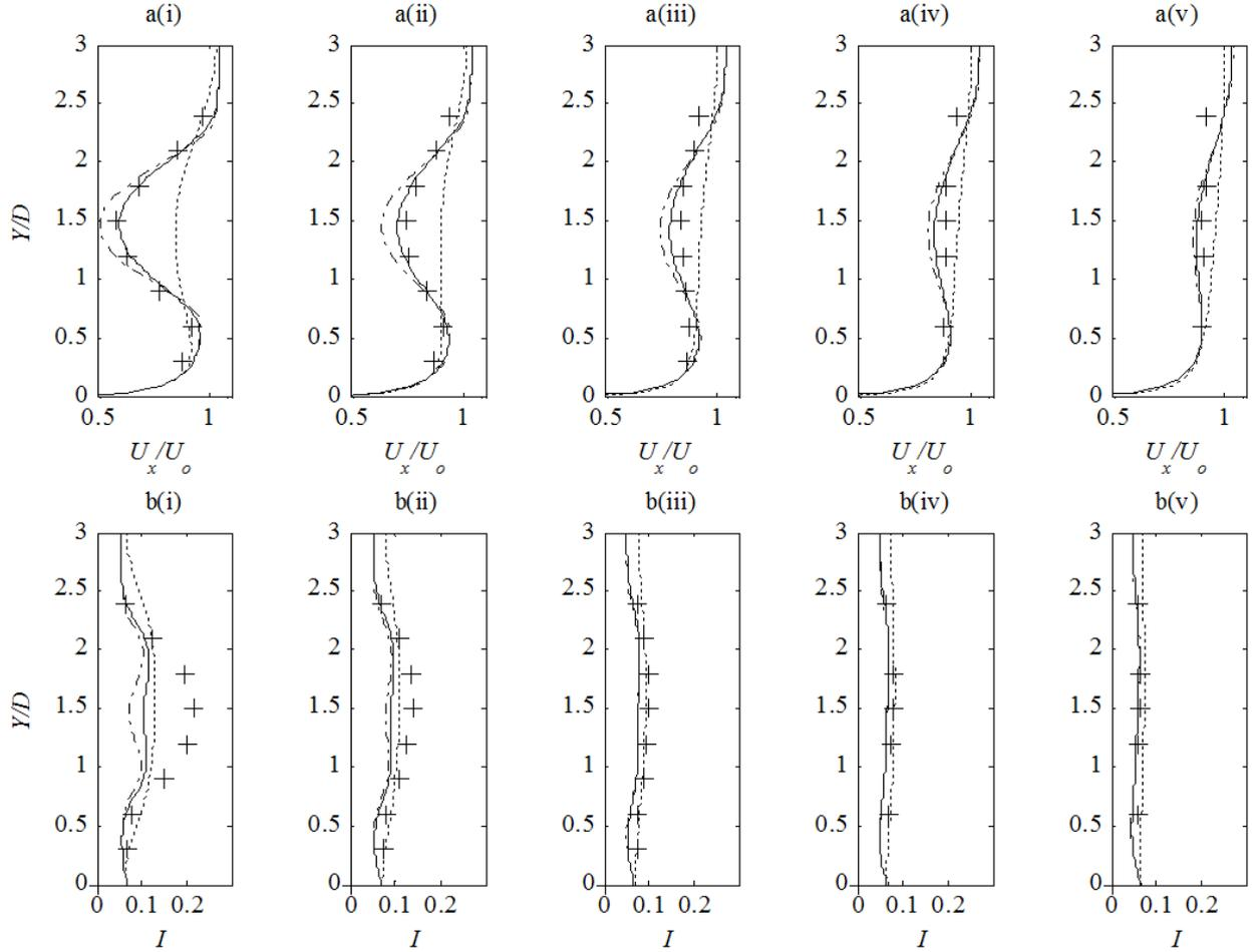
Figure 8 - Vertical velocity (a) and turbulence intensity (b) profiles for different turbulence source values.
