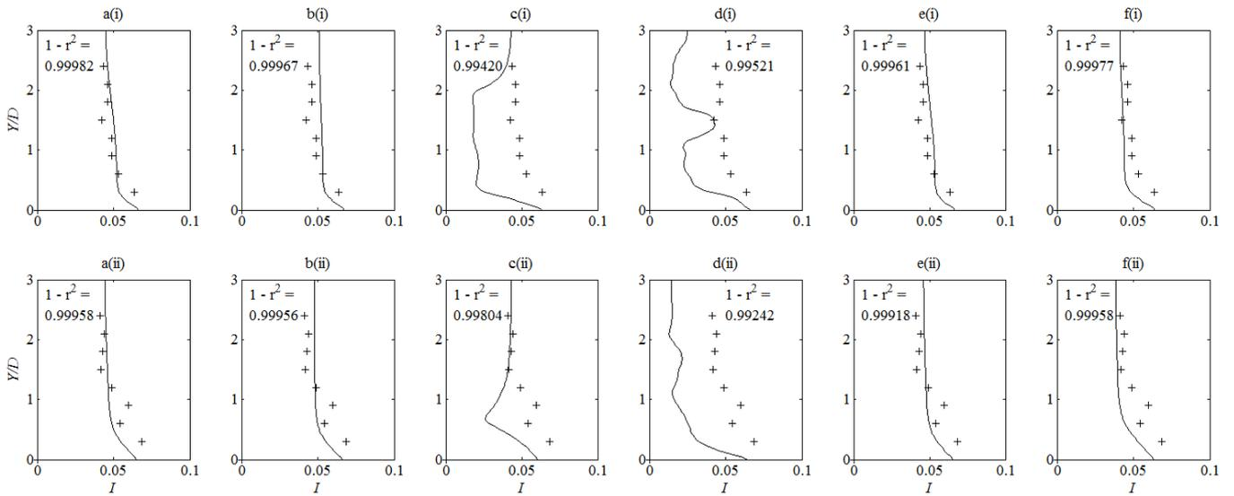
Figure 6 - Flume turbulence intensity. (i) 5 diameters upstream of disc position, (ii) 11 diameters downstream of disc position.
