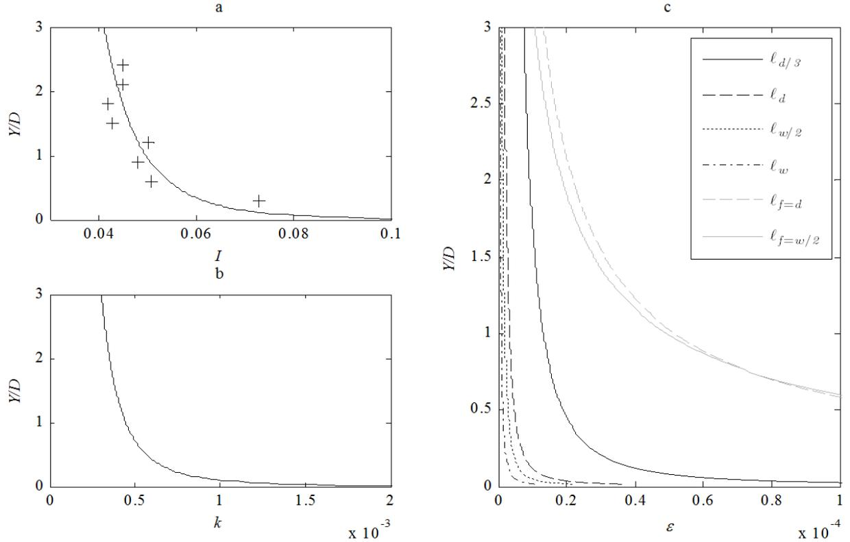
Figure 1 - Turbulence inlet parameters. a) turbulence intensity [crosses are experimental data, line is the fitted inlet profile, Equation 18], b) Turbulent kinetic energy, c) Turbulence dissipation for different turbulence length scales.
