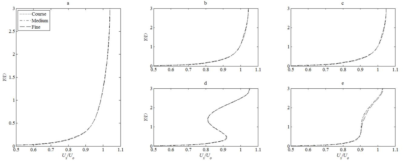
Figure 4 - Mesh Independence. a, b, and c are the flume results, d and e are the disc results. a is 5 diameters upstream of the disc position, b and d are 4 diameters downstream of the disc position, c and e are 11 diameters downstream of the disc position.
