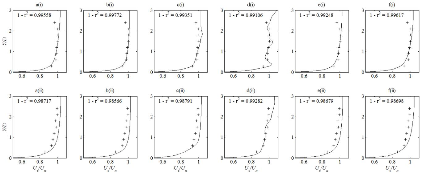
Figure 5 - Flume velocity profiles. (i) 5 diameters upstream of disc position, (ii) 11 diameters downstream of disc position.
