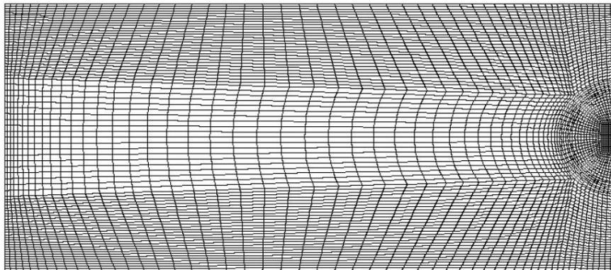
Figure 2 - Medium mesh on y-z plane showing disc to the right
