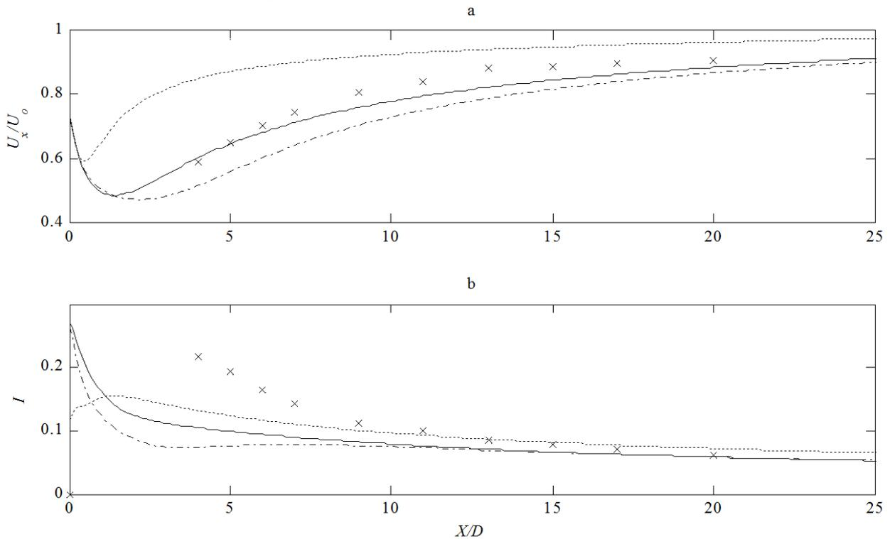
Figure 7 – Centreline velocity (a) and turbulence intensity (b) profiles for three disc turbulence source values:
