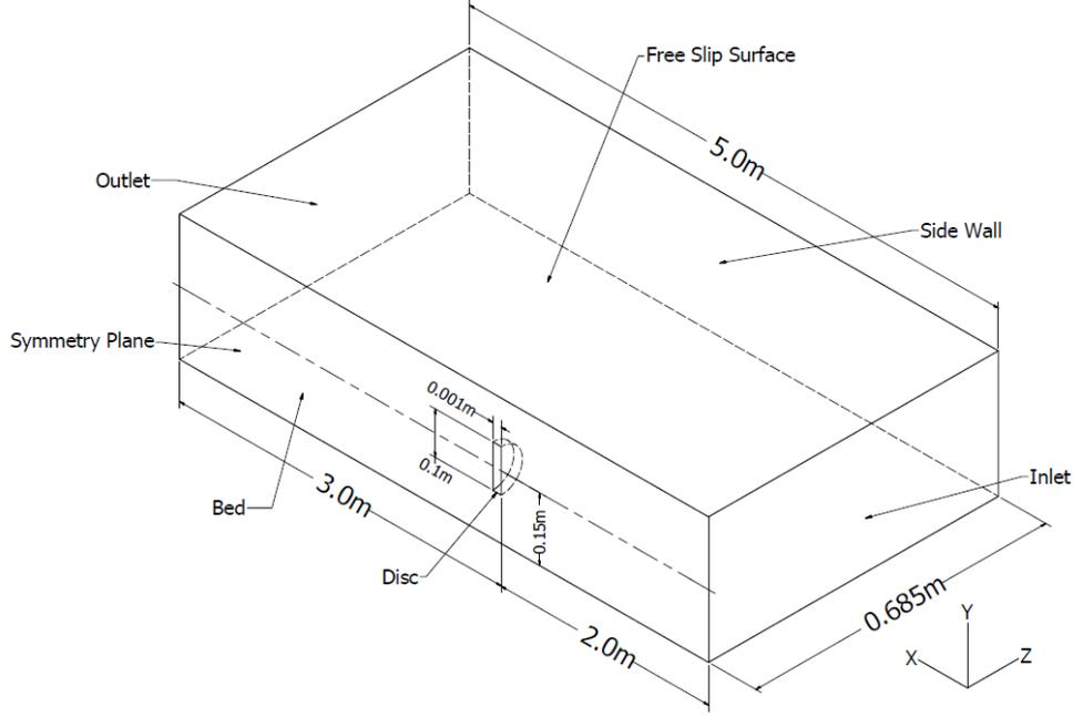
Figure 3 - Flow domain showing principle dimensions.
