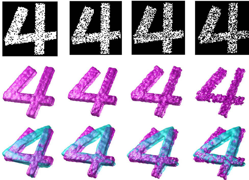
Figure 3.19: Top row: the target '4' contaminated by 30% (SNR=6.45dB), 50% (SNR=4.78dB), 70% (SNR=3.67dB), and 90% (SNR=2.75dB) level of noise from left to right (viewed from slice). In addition, the formula of SNR calculation can be found in appendix A. Middle row: the target '4' with noises viewed in 3-D. Bottom row: the registration results corresponding to the noise levels.
