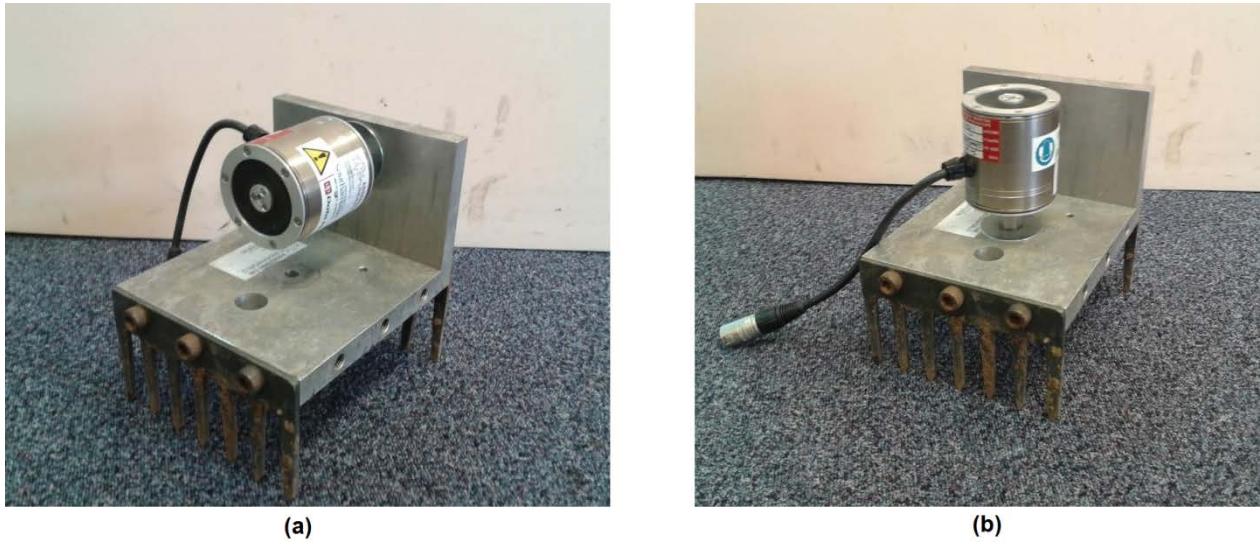
Figure 2: rectangular platform with shaker attached horizontally (a) and vertically (b)
