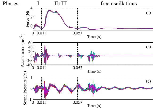
Figure 5. Force (a), acceleration (b) and sound pressure (c) recorded during 33 different keystrokes.
