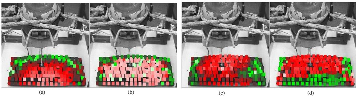
Figure 7. Mode of vibration at 61.25 Hz (a-b) and at 126.9 Hz (c-d) recorded by the Polytec laser scanning vibrometer. Velocity magnitude (a,c) and phase (b,d).
