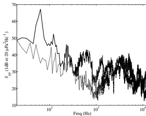
Figure 9. Sound pressure of the full keyboard (continuous line) and of the cut-out of Figure 8 (dotted line).
