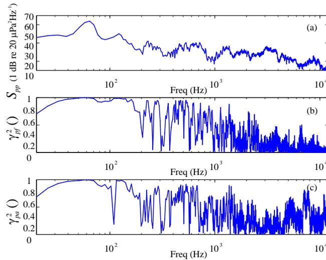
Figure 4. Noise emission ‘T’ key on Dell keyboard: (a) sound pressure PSD: (b) coherence between sound pressure and impact force: (c) coherence between sound pressure and key acceleration.
