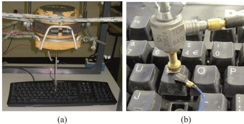
Figure 1. Apparatus setup (a) a shaker is used to tap the keyboard (b) key “I” and tip are instrumented
