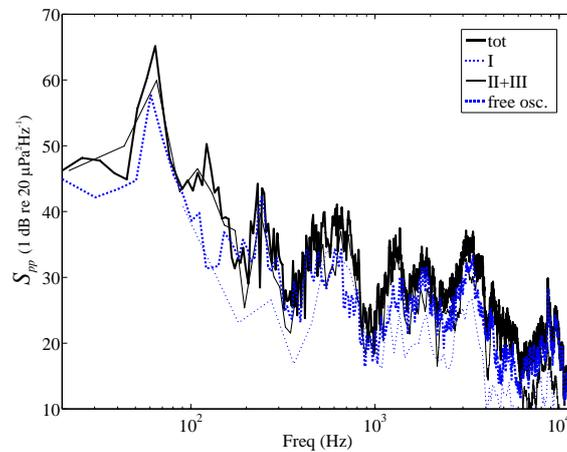
Figure 6. Sound pressure PSD for the full keystroke (thick solid black line) and for the periods I (thin dotted blue line), II+III (thin solid black line) and free oscillation (thick dotted blue line).
