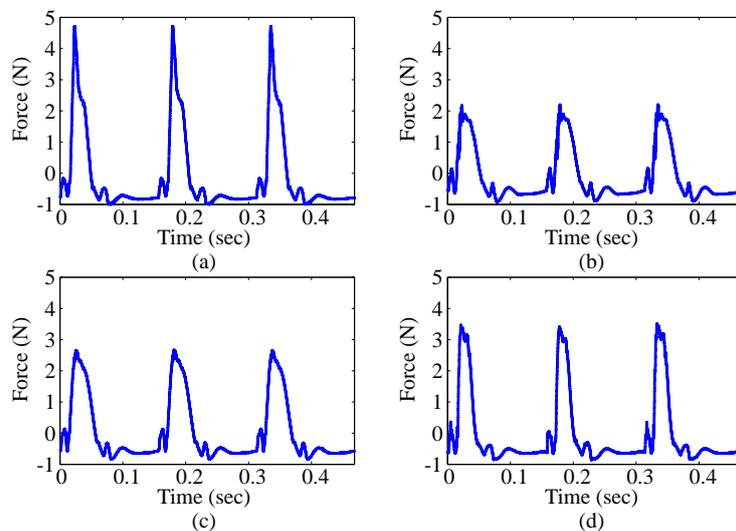
Figure 3. Tapping force histories for different tips while pressing a keyswitch with a 6.4 Hz sinusoid signal: 1mm foam (a) 2mm foam (b) 3mm foam (c) 2mm rubber (d).
