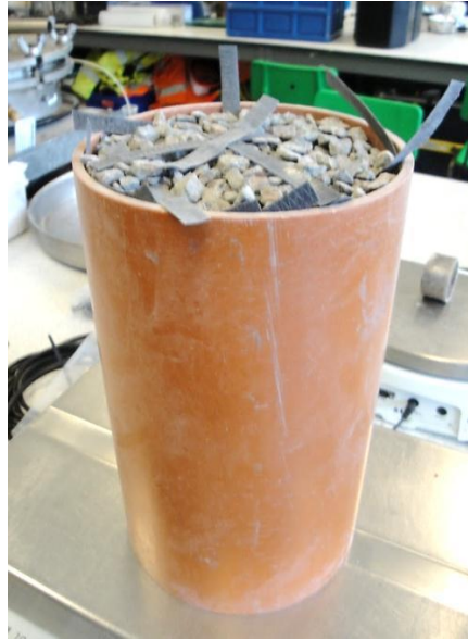
Figure 3.4: Cylindrical compaction mould used for the determination of the dry density of scaled ballast
