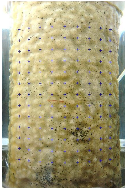
Figure 6.6: Typical captured image of a triaxial specimen during shear deformation showing measurement grids used for image-based deformation measurement
