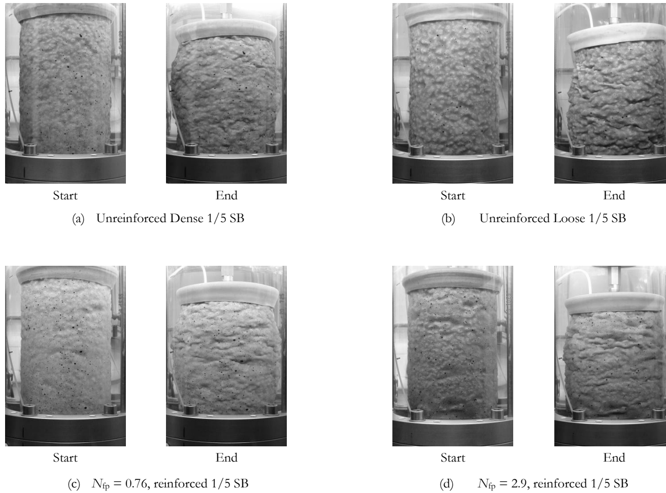
Figure 6.9: Photographs of triaxial specimens at the start and end of shear deformation carried out at 30 kPa cell pressure
