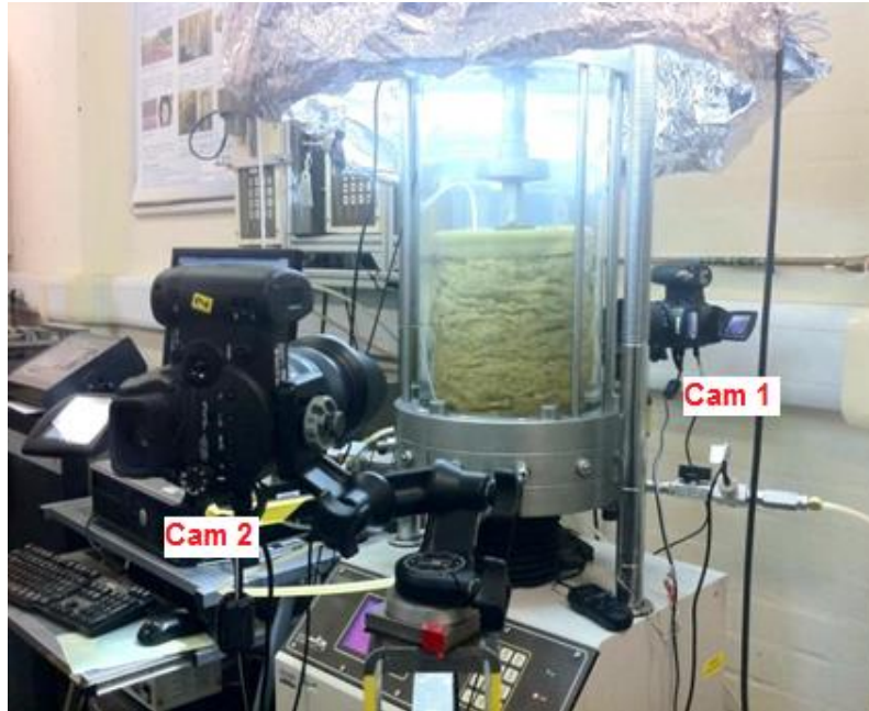
Figure 6.1: The triaxial setup for image-based deformation study showing the transparent cell, cameras, uniform light source and light reflecting curtain
