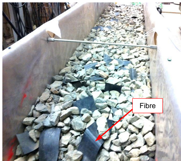
Figure 7.7: Fibre reinforced ballast layer in the test rig before compaction
