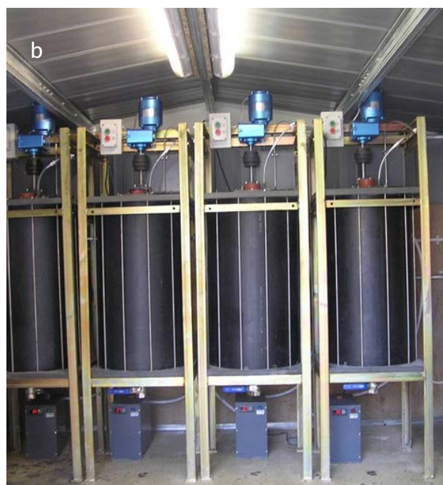
Fig. 15. 75-L CSTR digesters. a) Schematic showing b) four digesters image (1) NB port, (2) motor to propel the stirrer, (3) heater, (4) heating coil, (5) digestate outlet
