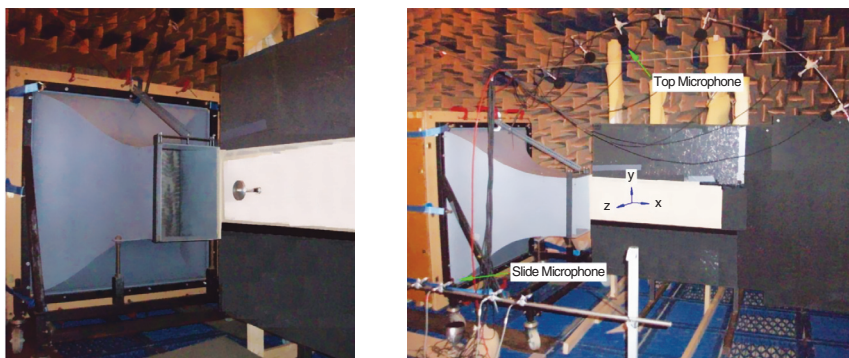
Figure 13: Experiment setup in the anechoic chamber.
