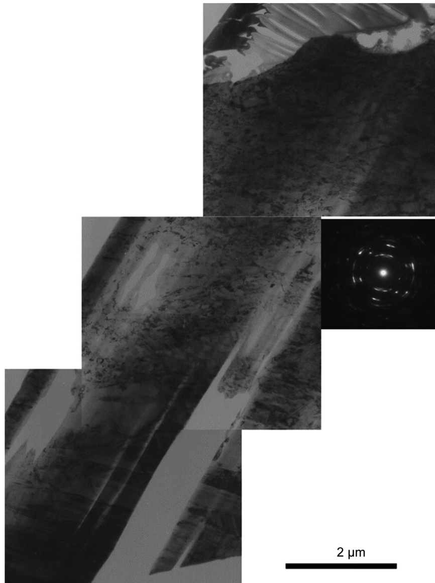
Fig. 3. A plan view bright field TEM cross-section image of Area 1 from Case 1 shows subsurface microstructure changes under the worn surface. Insert diffraction pattern suggests a nanocrystalline structure at the surface.
