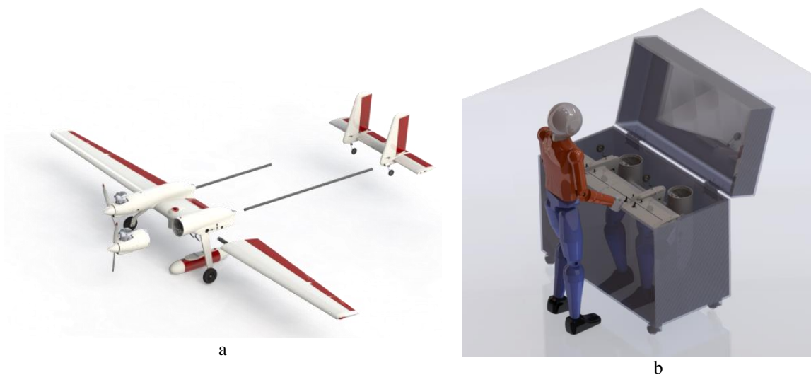
Figure 3 – (a) Spotter partly disassembled for transportation. (b) Spotter in the flight box
