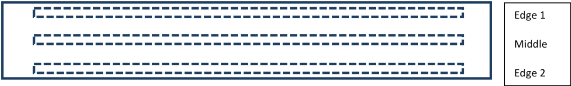
Figure 6: A diagram describing the method used to image the surfaces of the polymer slides. Images were taken along the length of each fluid channel following the three paths set out above as “Edge 1, Middle, and Edge 2.” Images were taken from left to right moving along the channel.
