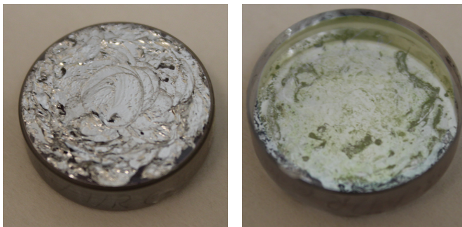
(a) Solder applied directly to the HR dielectric (b) View through the unsoldered surface
