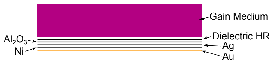
Figure 5.22: Sputtered layers applied to the base of the gain medium.
