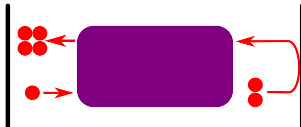
Figure 2.3: A flux of indistinguishable photons can be created by passing photons repeatedly through a gain medium
