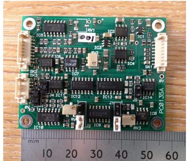
Figure 5: Sensor array interface circuit
