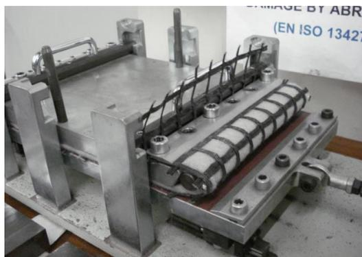
Figure 2. Equipment for the abrasion damage tests.
