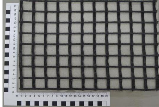
**Figure 1.** Composite tested (GTX+GGR).
