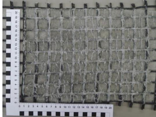
**Figure 3.** Specimen of the geocomposite after sequential mechanical and abrasion damage tests.
