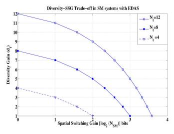
Fig. 1. Trade-off between transmit diversity and switching gain in SM systems employing EDAS with various number of transmit antennas.
