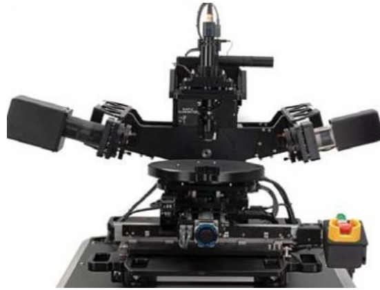
Figure 43 A Woollam ellipsometer.
