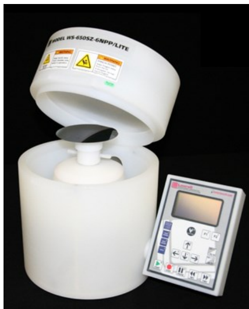
Figure 40 Spin coater used in this project (Laurell WS-650SZ-6NPP/LITE).
