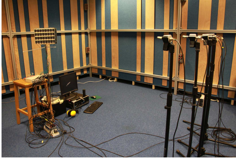
Figure 3.29: Set up of the measurements performed in a listening room.
