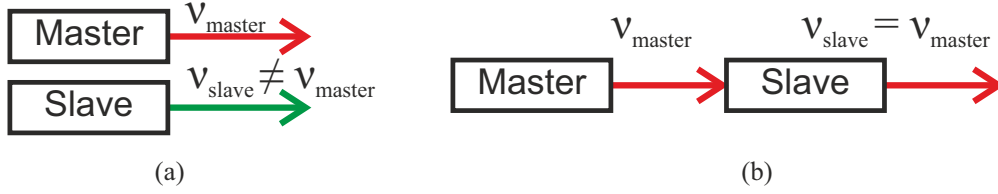
FIGURE 2.7: Optical injection locking: two lasers emitting at different frequencies (a) can be synchronised by injecting the signal from one laser into the other (b).
