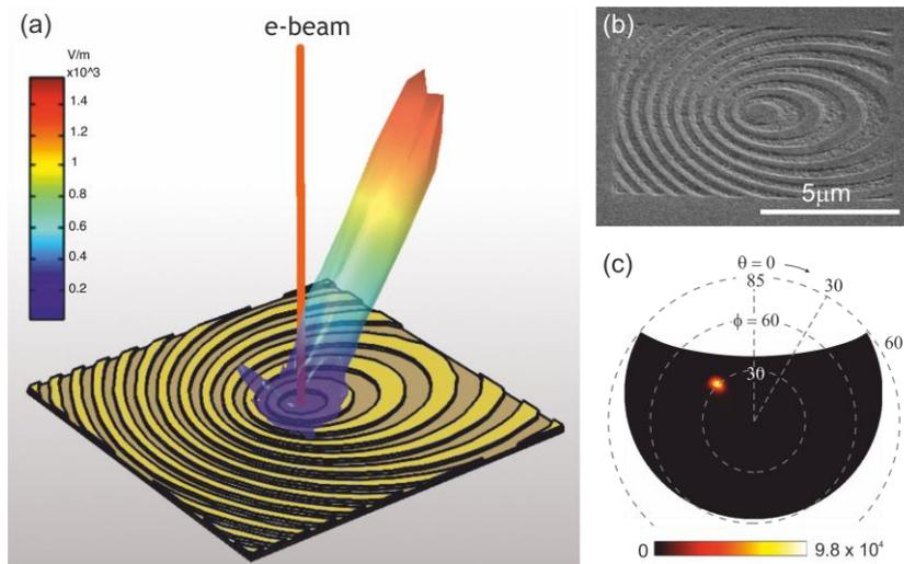
**Figure 1:** (a) Far-field radiation pattern from electron impact (modelled as a transition radiation dipole plus cylindrical surface plasmon wave) on a holographic mask designed to generate a plane wave at 30° to the surface normal. (b) Scanning electron microscope image of the above mask on a gold substrate. (c) Polar plot of 800 nm light emission from the above hologram mask [background unstructured gold emission subtracted].
