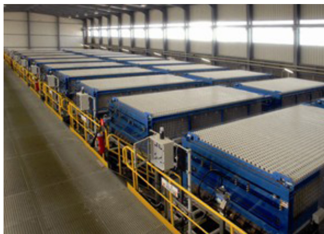
Fig. 4. A typical FM21-SP chlorine production cell room at Ineos ChlorVinyls, Runcorn, UK. The production rate is 10 to 30 ton day -1 with an energy consumption of 2200 Wh ton -1 . Further details are available in reference [37].
