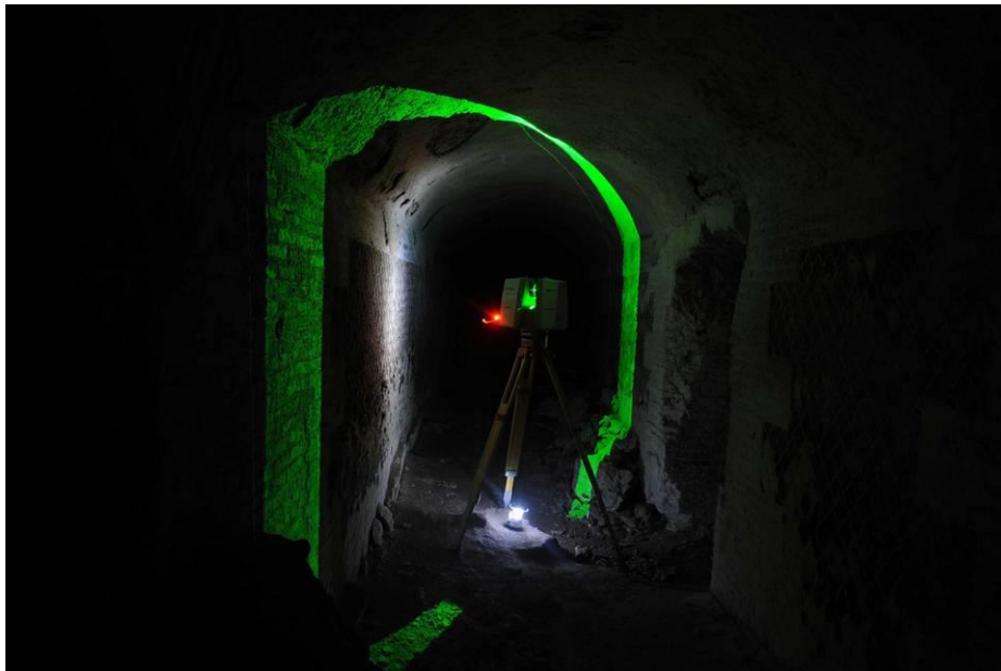
Figure 5.4 Using a time of flight laser to record the interior of a corridor at the Portus Project (Image author's own).
