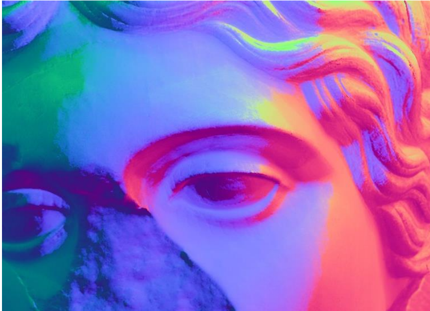
Figure 5.13 A normal map of the statue of a young woman derived from an RTI. The different colours in the image indicate the direction in which each pixel is sloping. This can be observed in the fact that the pixels on the left of the image are green while those on the right are cyan.(image author's own).
