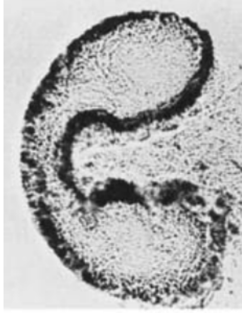
Figure 7.5 – This figure is taken from the paper by Haas and Sturtevant [73]. It shows a helium bubble after a 1.22 Mach shock has passed through. The bubble is surrounded by air at normal atmospheric pressure.
