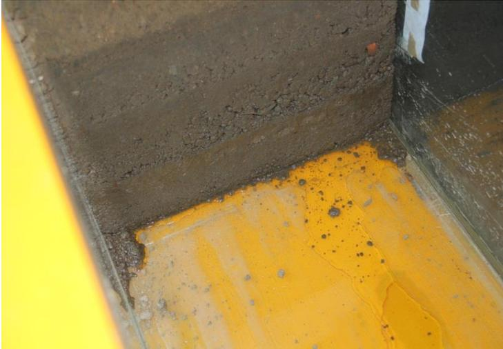
**Figure 5 – Layering of the soil after compaction, creating singularities.**
