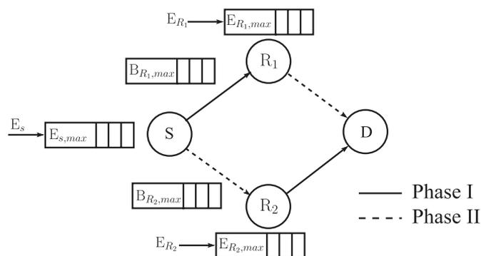
Fig. 1. Successive relaying network where EH nodes are equipped with finite buffer for both energy and data storage.
