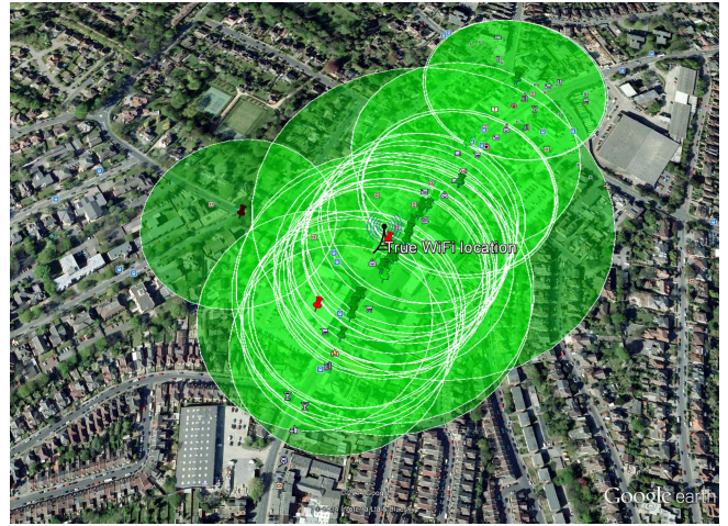
Figure 4: The reports for a sample Wi-Fi hotspots taken from the OpenSignal–Wi-Fi dataset with the true Wi-Fi hotspot position marked on the map. Each circle shows the value and the precision (2 standard deviations) reported by the user.
