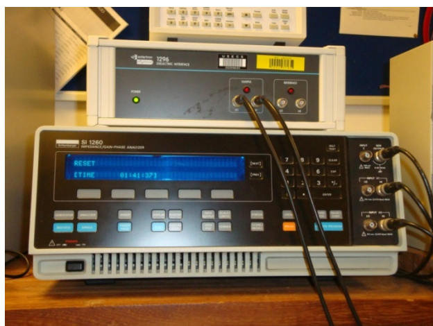
Fig. 3.2 Solartron 1296 dielectric interface and model 1260A impedance / gain- phase analyzer
