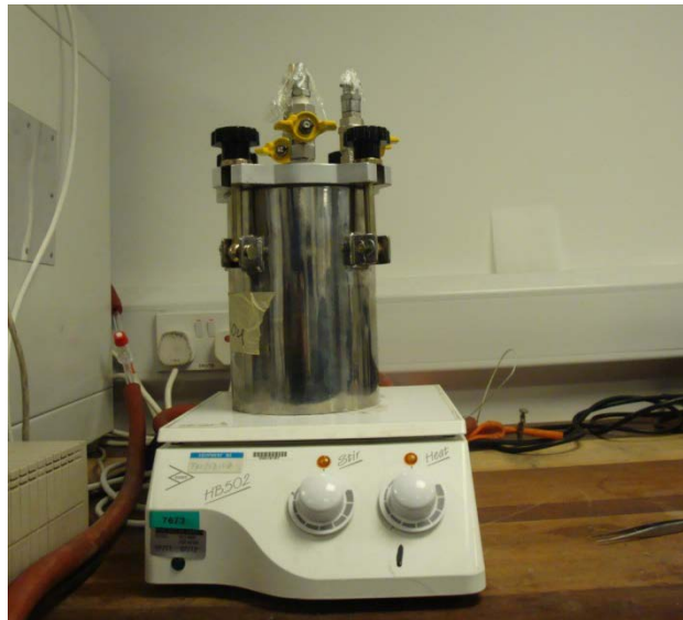
Fig. 2.3 Oil pre-treatment system
