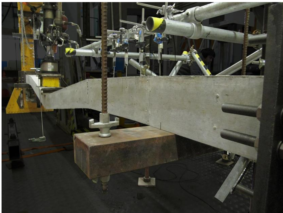
Figure A.6.7: Full view of loaded sample at end of CMA phase ( \delta=200\text{mm} ).
