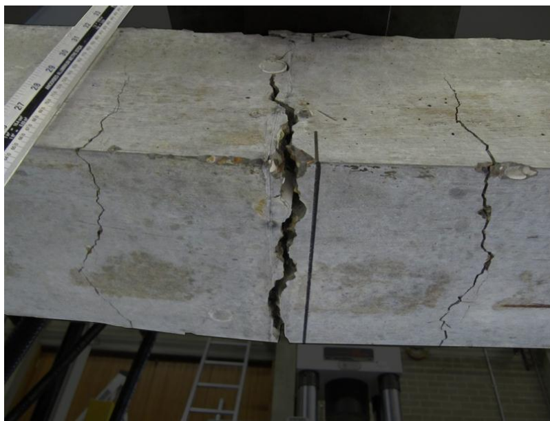
Figure A.6.6: Mid-span crack pattern of underside of sample at approximately H_{max} ( \delta=100\text{mm} ).
