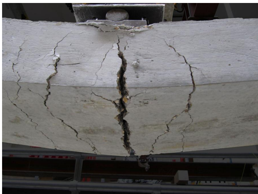
Figure A.6.4: Mid-span crack pattern of underside of sample at approximately end of CMA ( \delta=200\text{mm} ).
