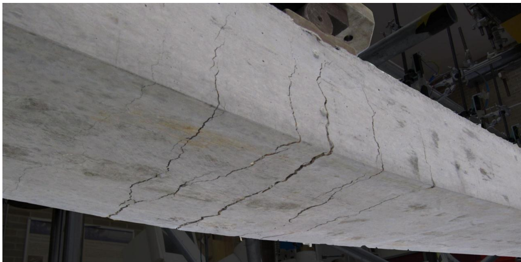
Figure A.6.2: Mid-span crack pattern of underside of sample at approximately H_{max} ( \delta=100\text{mm} ).
