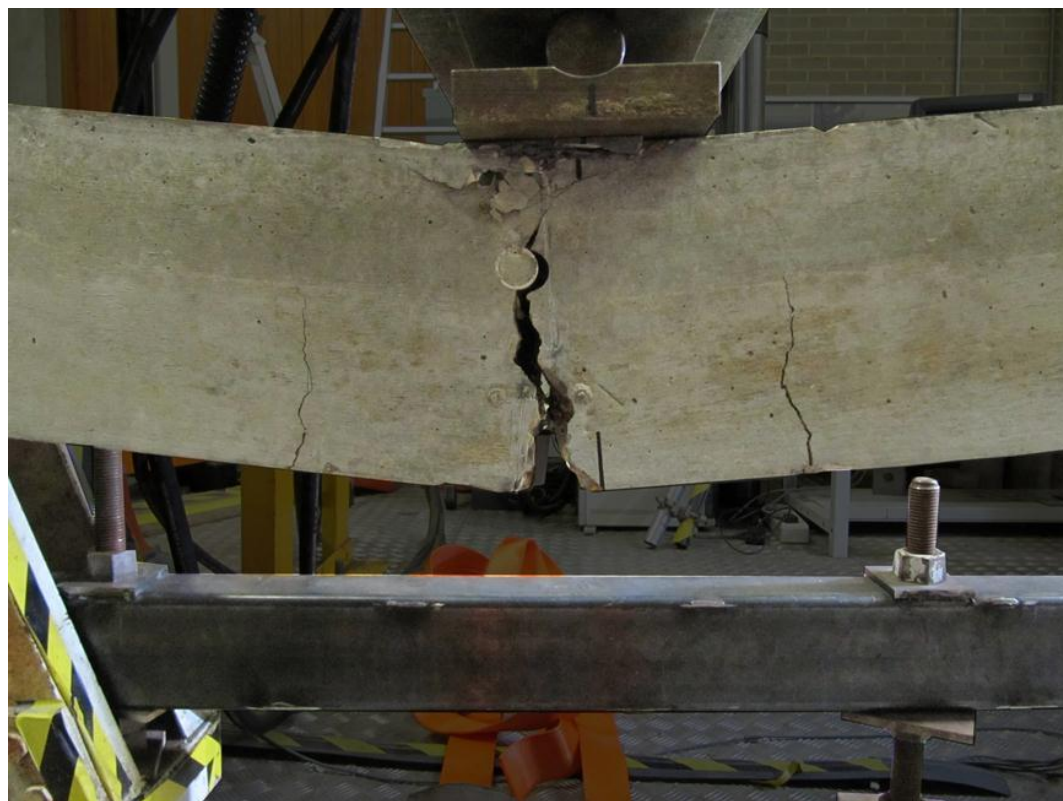
Figure A.6.9: Mid-span crack pattern of underside of sample at approximately end of CMA ( \delta=200\text{mm} ).
