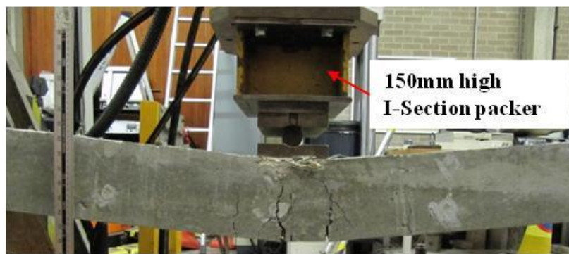
Figure 3.27: 150mm steel I-Section packer to the load actuator
