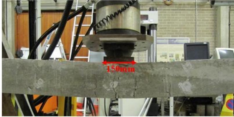
Figure 3.25: Loading arrangement at the centre of the specimen
