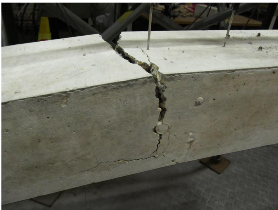
Figure A.6.8: Crack pattern at support C at approximately end of CMA ( \delta=200\text{mm} ).
