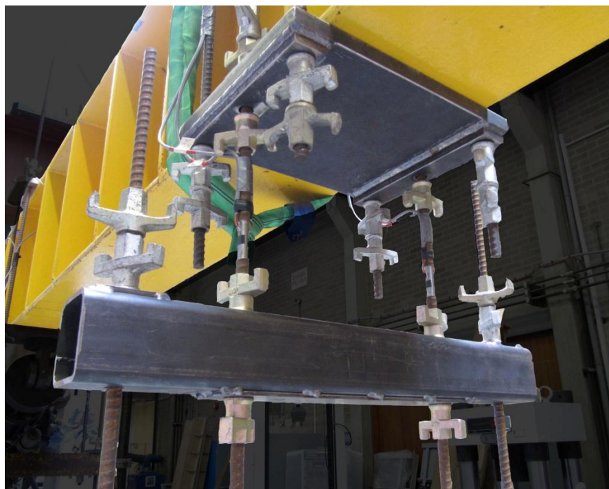
Figure A.1.5: Hanger Detail with strain gauges.
