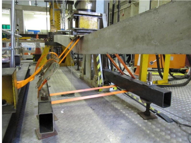
Figure 3.26: Strapping down arrangement at the limit of the actuator's stroke
