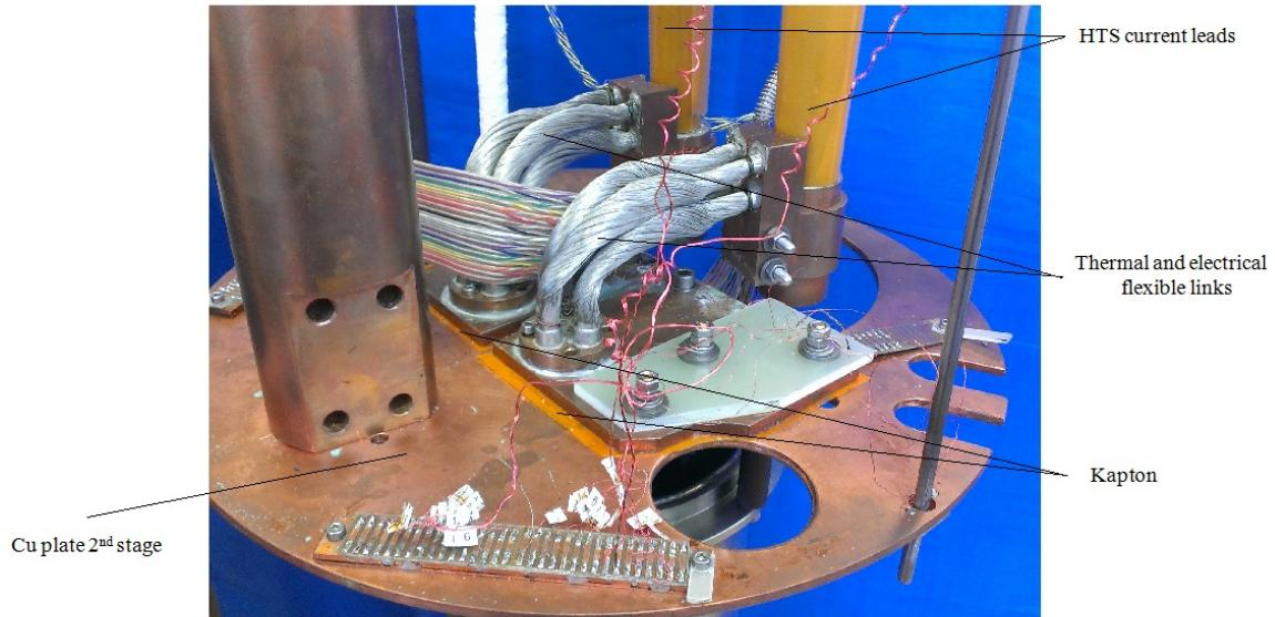
**Figure 2.7:** Thermal and electrical flexible links.
