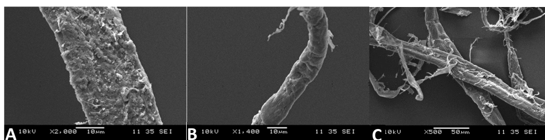
Figure 5.2-6. SEM images of 1% NaOH extracted dried milled MSW pulp.
