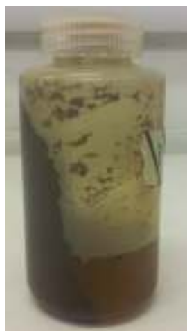
Figure 6.6-3. Image of centrifuged hydrolysate showing the concentrated sugar solution separated from the residual solid after centrifugation.
