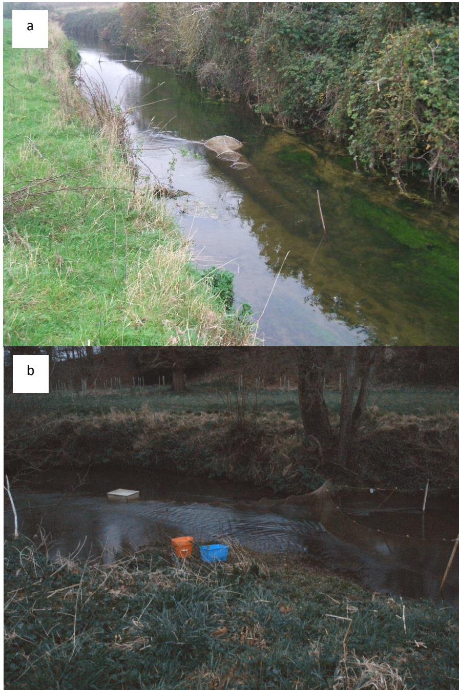
Fig. 4.7. Winged fyke nets with entrances facing upstream to catch (a) adult European eels 0.5 km upstream of Tide Gate 1 in the River Stiffkey, UK, and (b) sea trout smolts in the River Blackwater, UK, using a fine mesh catch box at the distal end.
