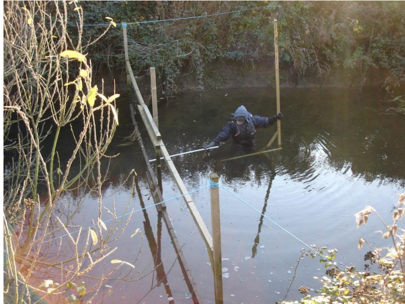
Fig. 4.2. Manual testing of a PIT loop (PL) located 65 m upstream from Tide Gate 1 in the in the River Stiffkey, UK.
