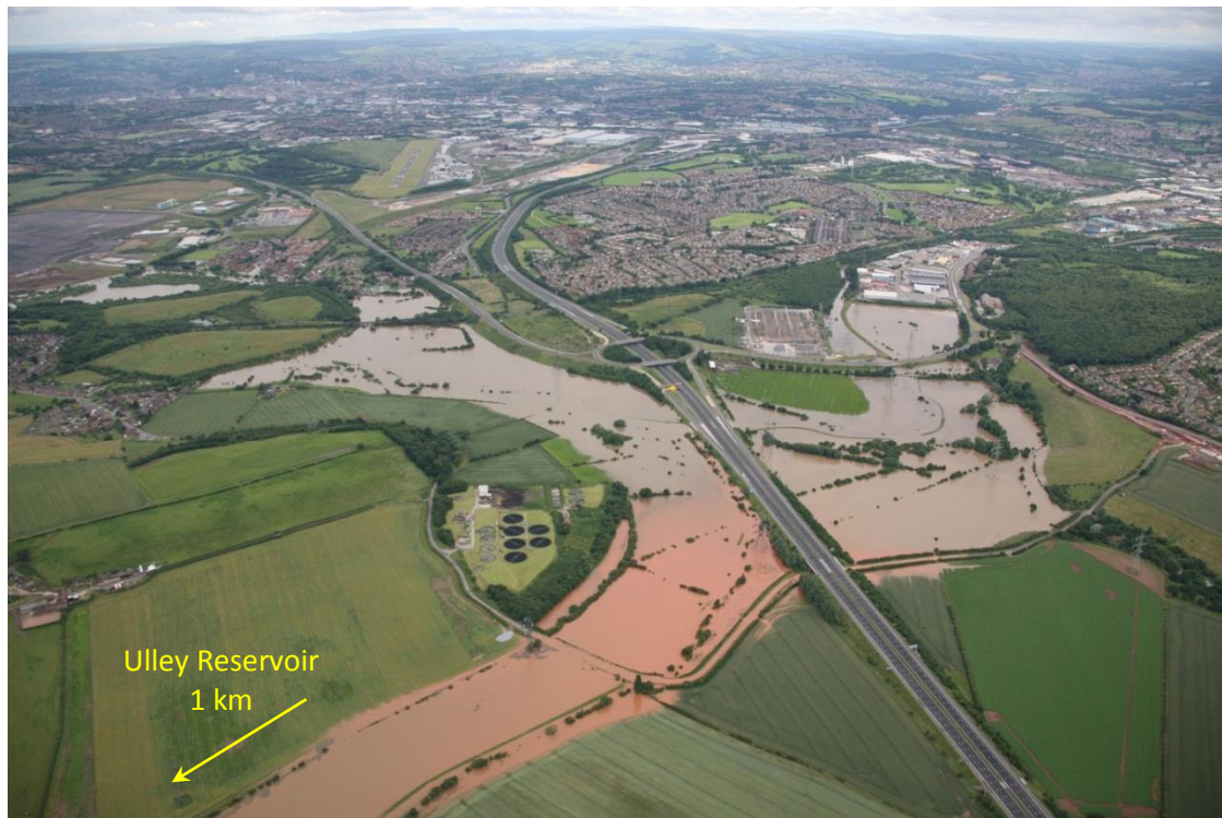
Figure 4.3 Aerial photograph (08:23 26/07/2007) showing antecedent flood extent on Ulley Brook and the River Rother (M1 junction 33 image centre). Red flood water discolouration caused by suspended sediment from Ulley embankment erosion (upstream) Photograph: Hinks and Mason (2007)
