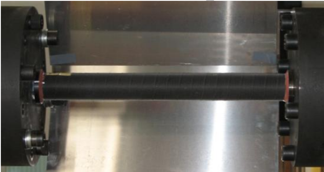
Figure 5: Test specimen mounted on the test machine with the two metal mirrors. Rotated view.
