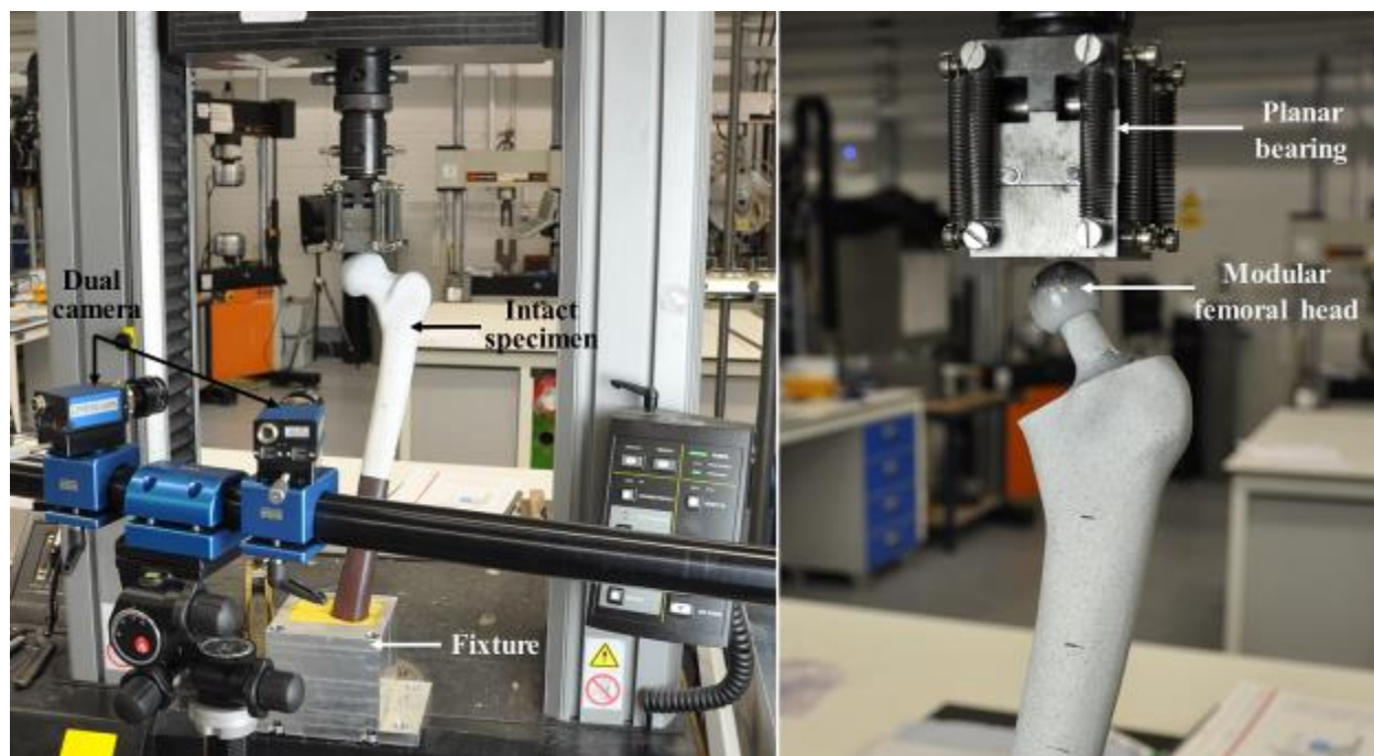
FIGURE 2: The experimental set-up for DIC measurement along with the planar bearing: ( left ) intact; ( right ) implanted.
