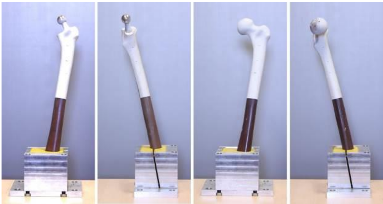
FIGURE 1: The position and orientation of the tested femur specimens: tilted 10^\circ laterally in the frontal plane for both (a) implanted and (c) intact femur; dorsally by 10^\circ in the sagittal plane for both (b) implanted and (d) intact femur specimens.
