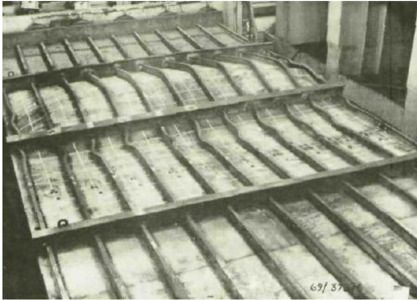
Figure 7 – Smith [9] Grillage Experiment Case 3a Failure Condition
