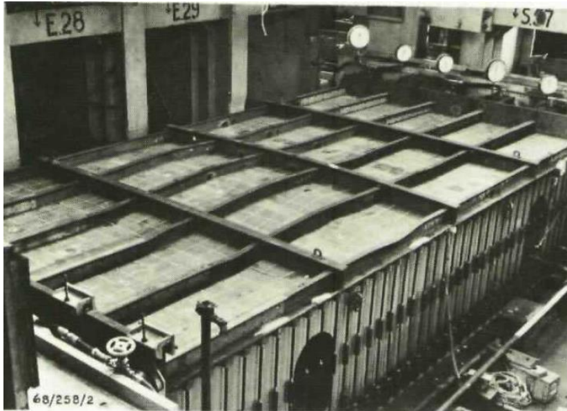
Figure 11 - Smith [9] Grillage Experiment Case 5 Failure Condition
