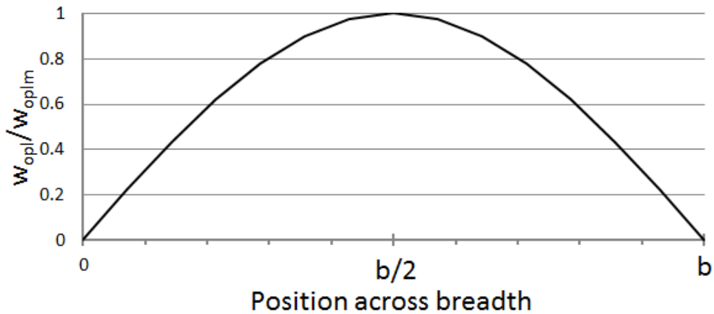
Figure 3: Example plate imperfection shape across breadth between longitudinal stiffeners at a/2
